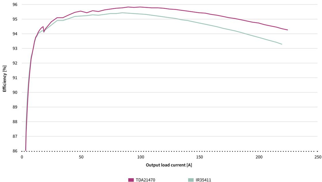
Efficiency levels at  $f_{sw} = 500$  kHz,  $V_{in} = 12$  V,  $V_{out} = 1.82$  V, five-phase measurement
