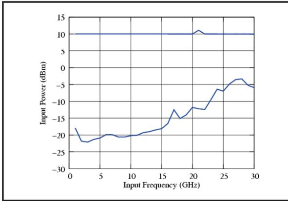
**Return Loss of Differential Output Ports**
