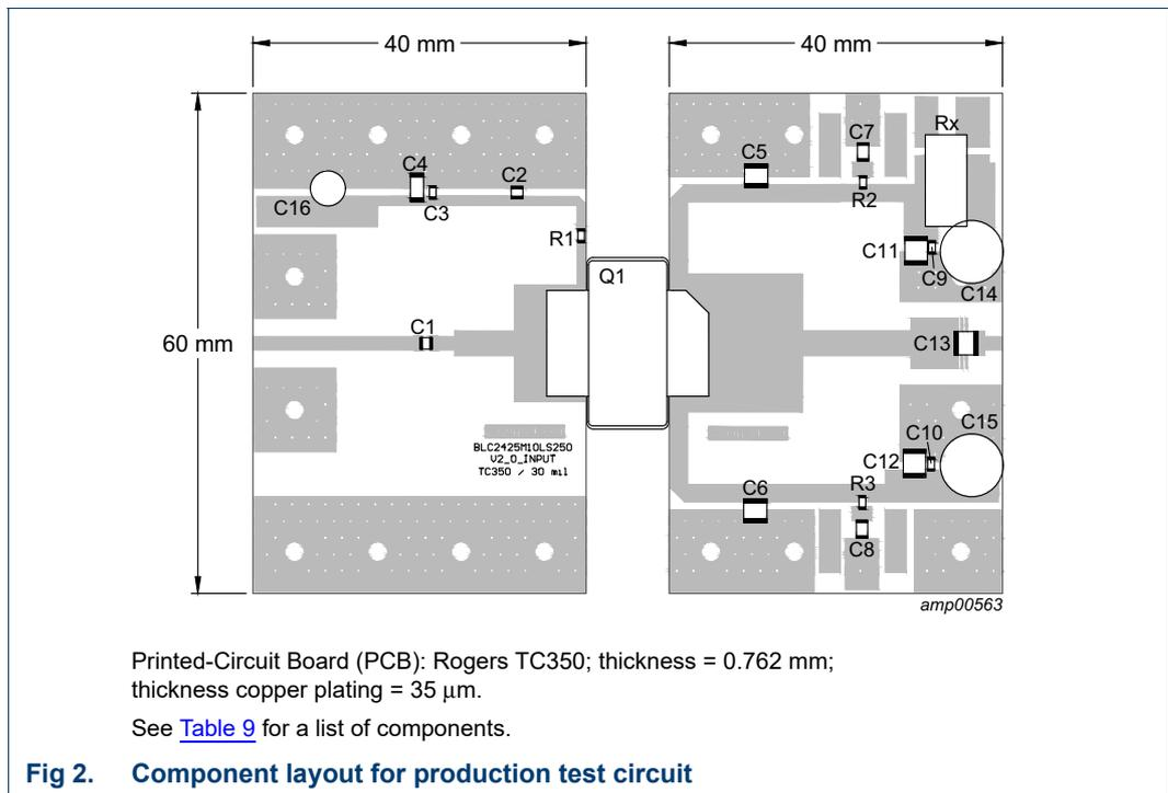
Printed-Circuit Board (PCB): Rogers TC350; thickness = 0.762 mm; thickness copper plating = 35 μm.
