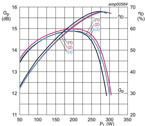
$V_{DS} = 32\text{ V}; I_{Dq} = 10\text{ mA}.$
