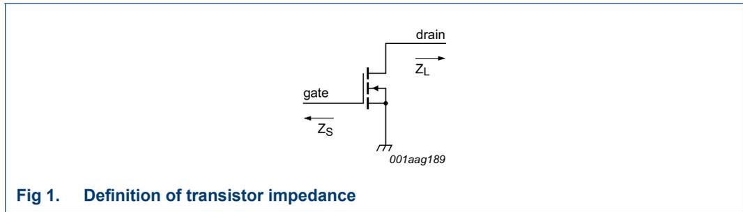
Fig 1. Definition of transistor impedance
