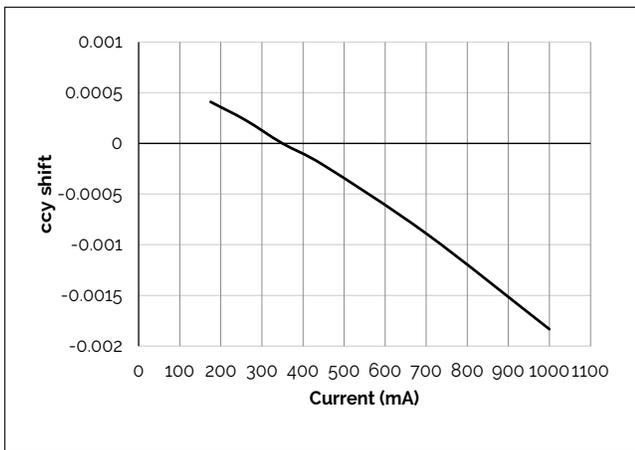
**Figure 10: V13C Drive Current vs. ccx Shift**
