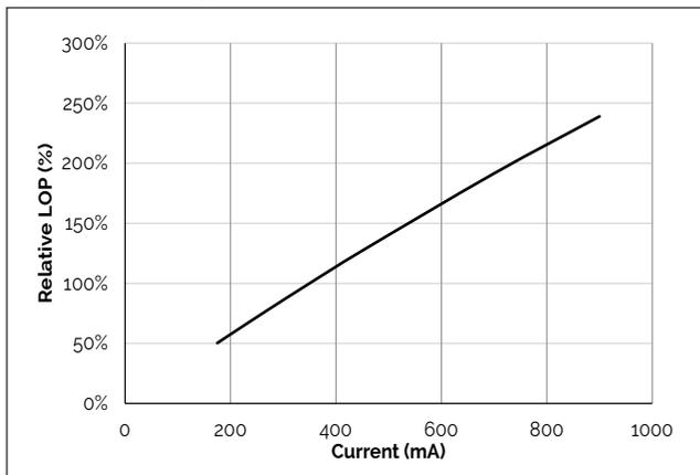
**Figure 4: V13C Typical Relative Flux vs. Current**
