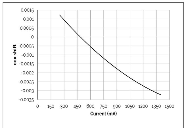
**Figure 11: V13C Drive Current vs. ccy Shift**
