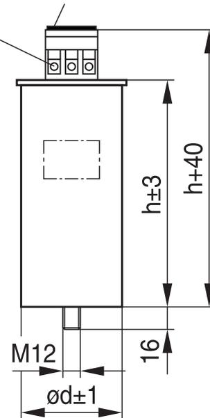
Torque = 10 Nm, Toothed washer J12 DIN 6797, Hex nut BM 12 DIN 439
