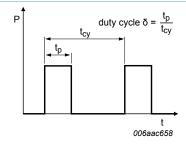
Fig. 9. Duty cycle definition
