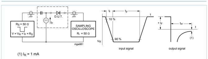
Fig. 8. Reverse recovery time: test circuit and waveforms
