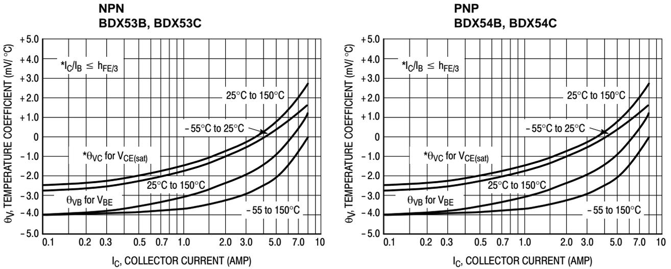
Figure 11. Temperature Coefficients
