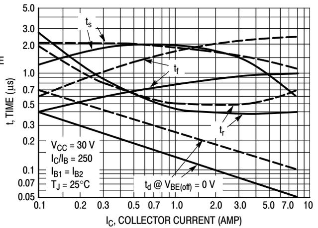
Figure 3. Switching Times
