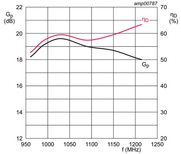
$V_{DS} = 51.6 \text{ V}$ ;  $I_{Dq} = 100 \text{ mA}$ ;  $P_L = P_{L(1dB)} (>1050 \text{ W})$ ;
