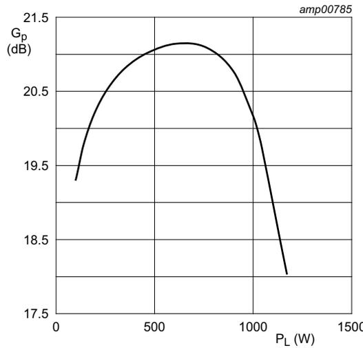
$V_{DS} = 50$  V;  $I_{Dq} = 200$  mA;  $t_p = 2.4$  ms;  $\delta = 6.4$  %.
