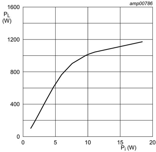
$V_{DS} = 50 \text{ V}$ ;  $I_{Dq} = 200 \text{ mA}$ ;  $t_p = 2.4 \text{ ms}$ ;  $\delta = 6.4 \%$ .
