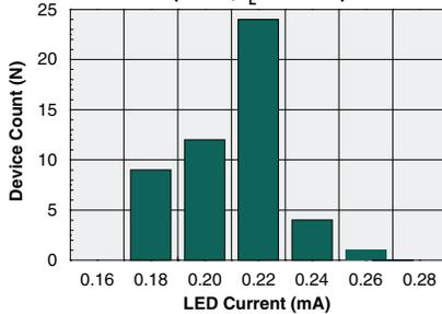
**Typical  $I_F$  for Switch Dropout**
