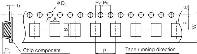
● Taping Reel Dimensions in mm (not to scale)
