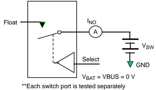
Figure 6. Power Off Leakage ( $I_{off}$ )
