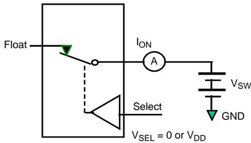
Figure 5. On Leakage
