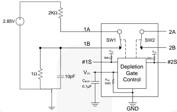
**Figure 4.  $t_{ON}/t_{OFF}$ ,  $t_{ONS}/t_{OFF}$**
