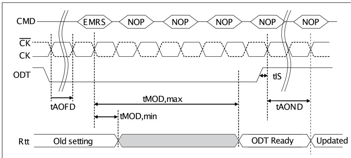
**ODT On/Off Timing for Active/Standby mode**
