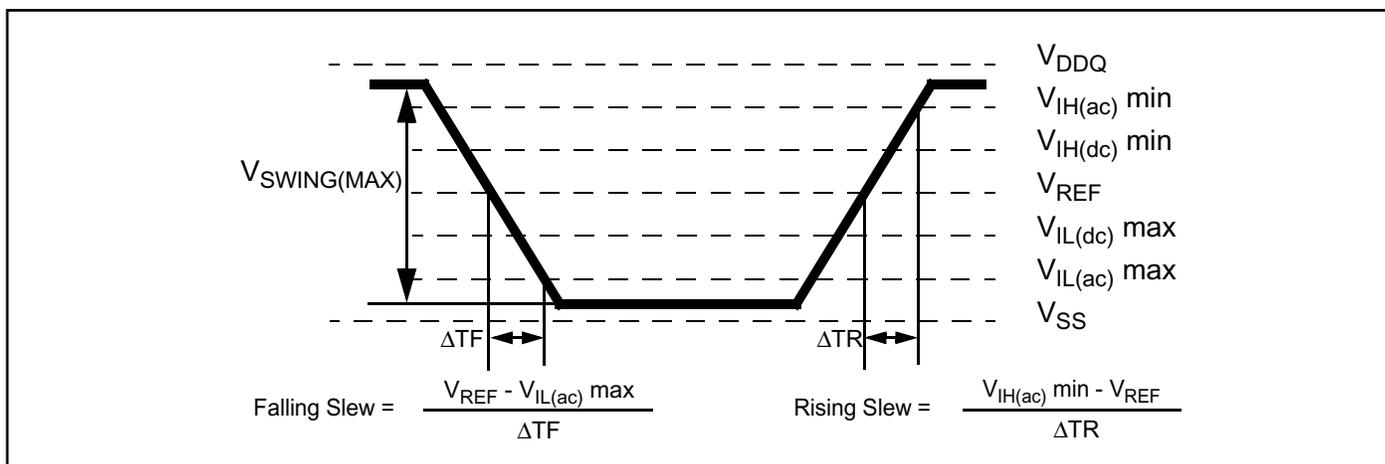
**Differential input AC Logic Level**
