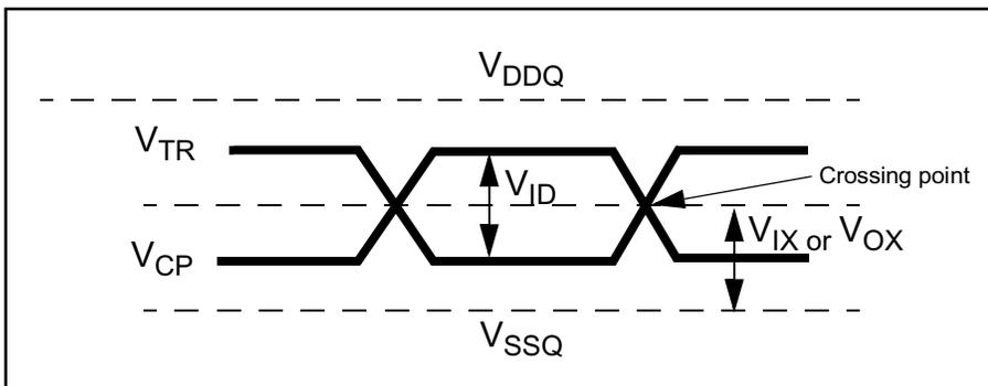
**Differential AC Output Parameters**
