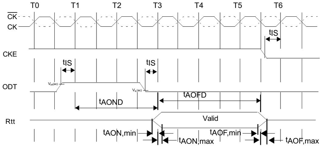
**ODT On/Off Timing for Power-Down mode**
