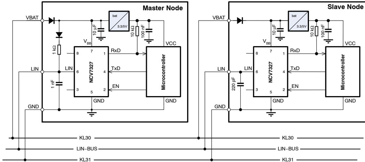
Figure 2. Typical Application Diagram for a Master Node
