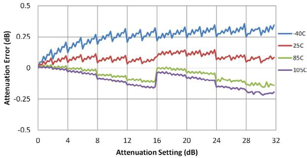
**Figure 26. Attenuation Error @ 1800 MHz vs. Temperature**
