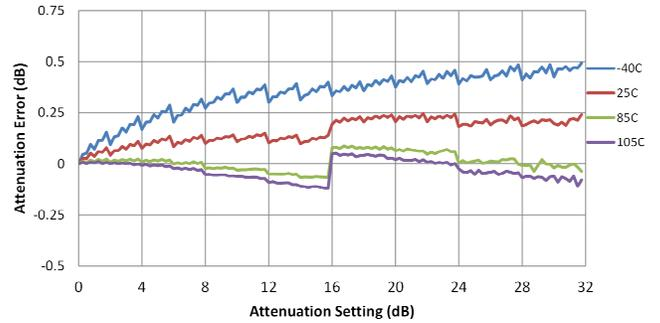
**Figure 27. Attenuation Error @ 3000 MHz vs. Temperature**
