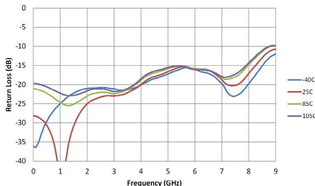
**Typical Performance Data @ 25°C and V<sub>DD</sub> = 3.3V unless otherwise specified**
