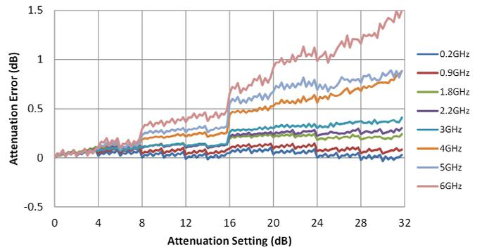
**Typical Performance Data, 0.5 dB Step @ 25°C and  $V_{DD} = 3.3V$  unless otherwise specified**
