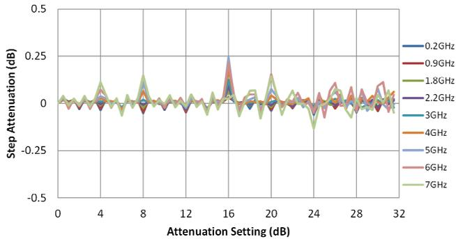
\* Monotonicity is held so long as step-attenuation does not cross below -0.5 dB
