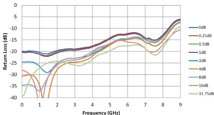
Figure 21. Input Return Loss vs. Temperature for 16 dB Attenuation Setting
