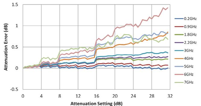
**Typical Performance Data, 1 dB Step @ 25°C and  $V_{DD} = 3.3V$  unless otherwise specified**
