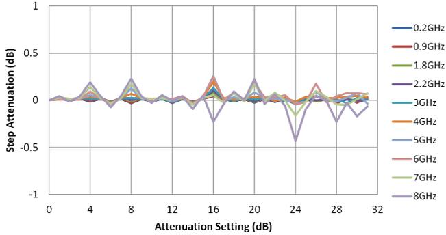
\* Monotonicity is held so long as step-attenuation does not cross below -1.0 dB
