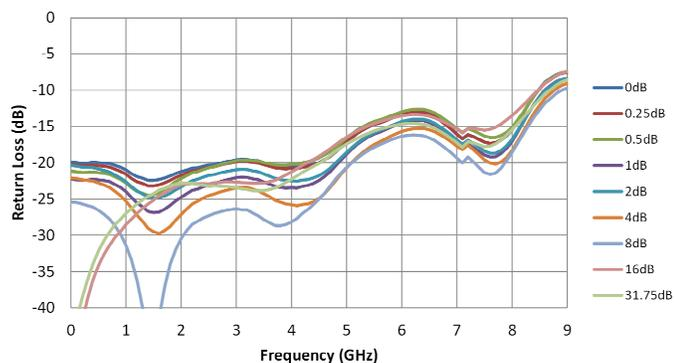
Figure 20. Output Return Loss vs. Attenuation Setting
