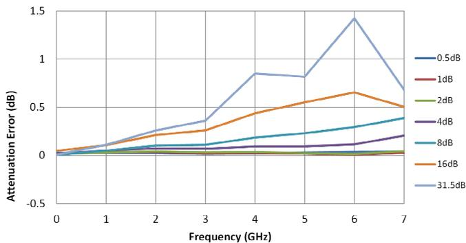
**Figure 13. 0.5 dB Attenuation Error vs. Frequency**
