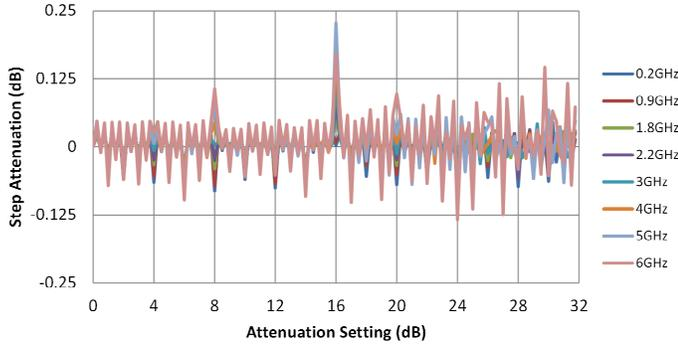
\* Monotonicity is held so long as step-attenuation does not cross below -0.25 dB
