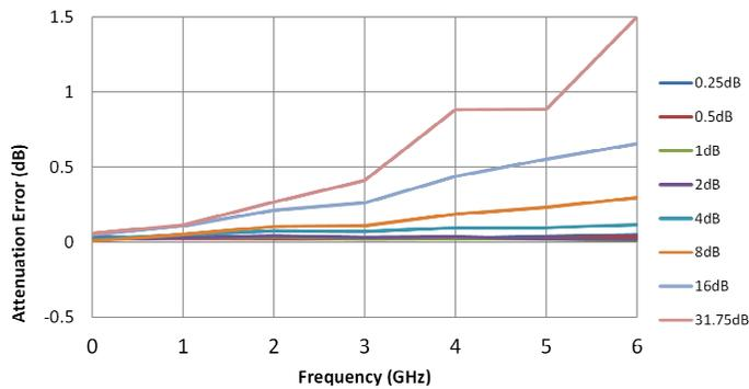
**Figure 9. 0.25 dB Attenuation Error vs. Frequency**
