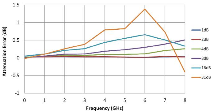
**Figure 17. 1 dB Attenuation Error vs. Frequency**
