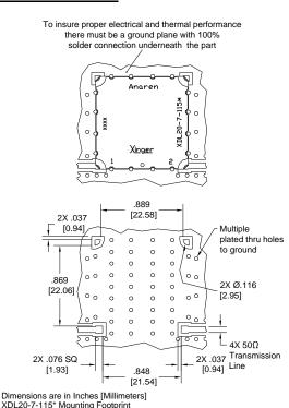
In order for Xinger surface mount delay lines to work optimally, there must be  $50\Omega$  transmission lines leading to and from all of the RF ports. Also, there must be a very good ground plane under the part with a number of plated thru holes to insure proper electrical performance. If any of these conditions are not satisfied, insertion loss, average delay and VSWR may not meet published specifications.
