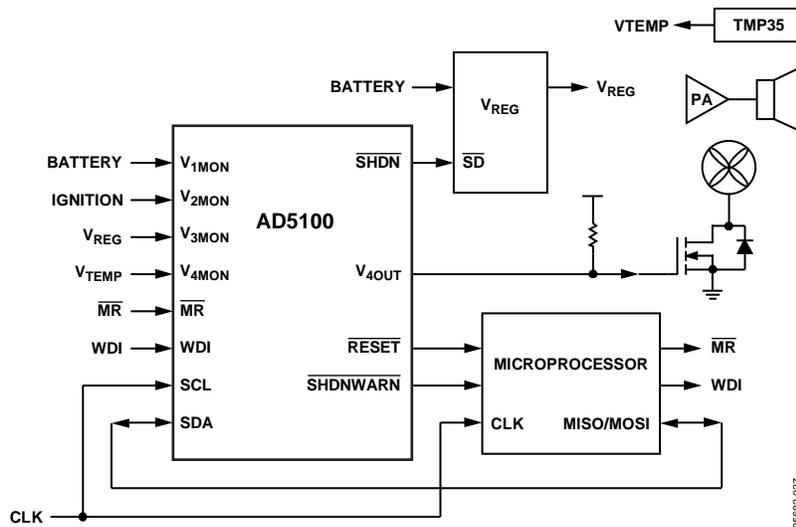
Figure 26. Power Amp Monitoring and Fan Control
