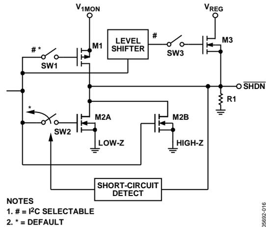
Figure 16. Shutdown Output
