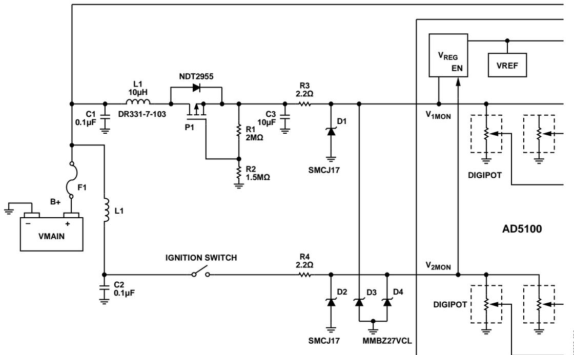
Figure 19. Protection Circuits
