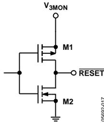
Figure 17. Reset Output
