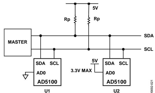
Figure 20. Two AD5100 Devices on One Bus
