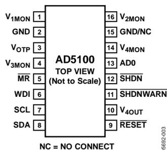
Figure 3. Pin Configuration
