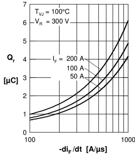
Fig. 2 Typ. reverse recov. charge  $Q_r$  versus  $-di_F/dt$
