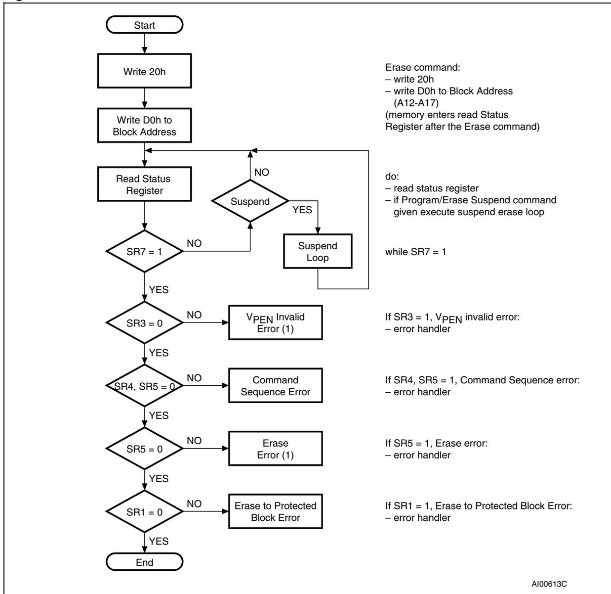
Note: 1. If an error is found, the Status Register must be cleared (Clear Status Register Command) before further Program or Erase operations.
