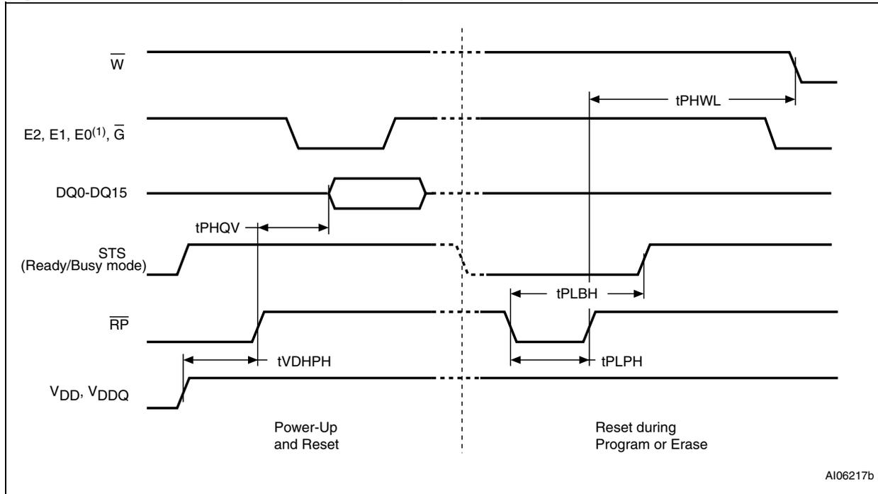
Note: 1.  $V_{IH}$  = Device Disabled (first edge of E0, E1 or E2),  $V_{IL}$  = Device Enabled (first edge of E0, E1 or E2). Refer to Table 2. for more details.
