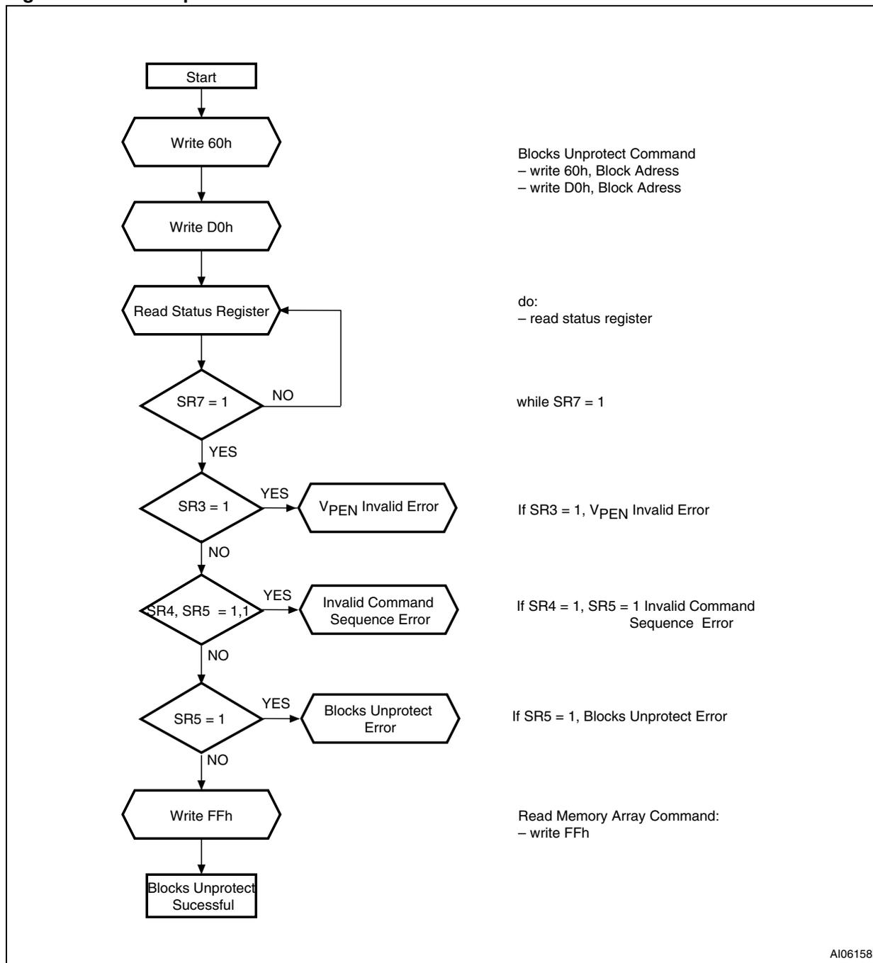
Figure 22. Protection Register Program Flowchart and Pseudo Code
