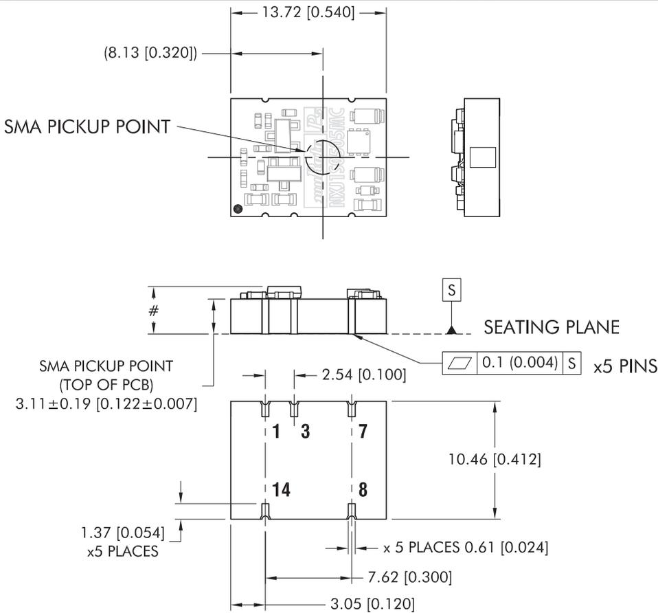
All dimensions in mm (inches), Controlling dimension is mm. Tolerances (unless otherwise stated)  $\pm 0.2$  (0.008). Components shown for reference only
