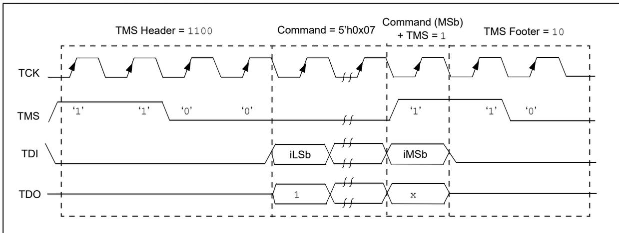
**FIGURE 6-4: SendCommand 2-WIRE (4-PHASE)**
