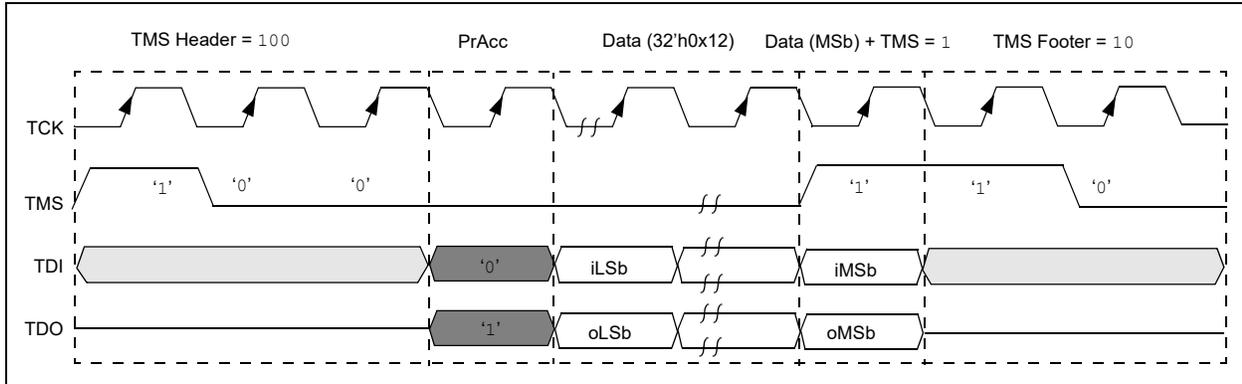
FIGURE 6-8: XferFastData 2-WIRE (2-phase)
