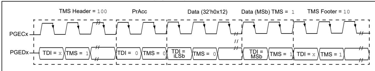
**FIGURE 6-9: XferFastData 2-WIRE (4-PHASE)**
