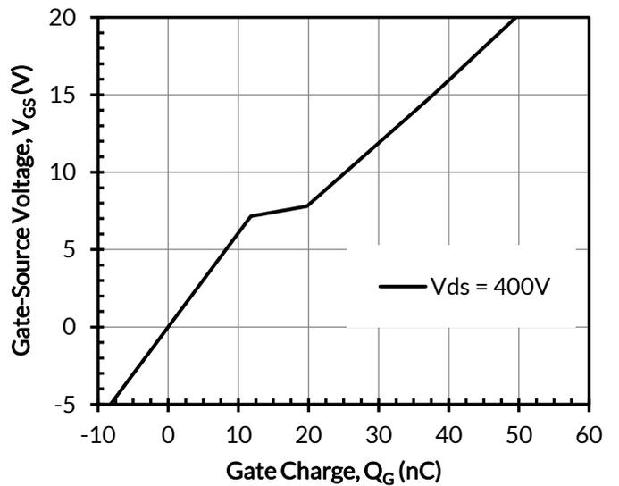
Figure 8. Typical gate charge at  $I_D = 40A$
