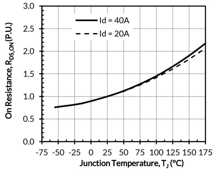
Figure 4. Normalized on-resistance vs. temperature at  $V_{GS} = 12\text{V}$
