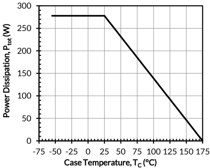
Figure 15. Total power dissipation
