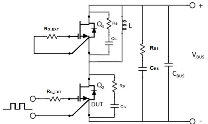
Figure 24. Schematic of the half-bridge mode switching test circuit with device RC snubbers ( $R_S = 10\Omega, C_S = 200\text{pF}$ ) and a bus RC snubber ( $R_{BS} = 2.5\Omega, C_{BS} = 100\text{nF}$ ).
