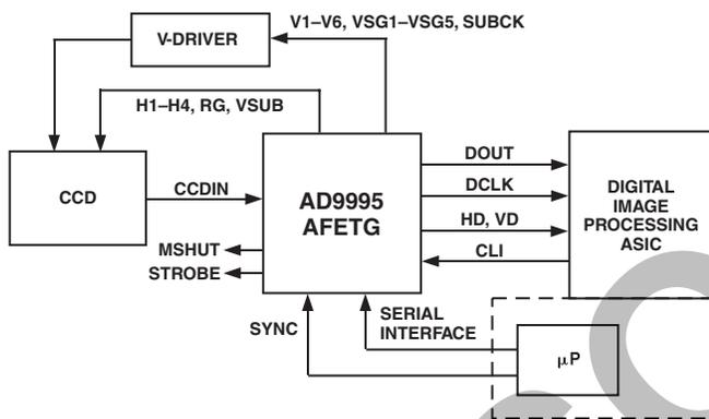
Figure 1. Typical System Block Diagram, Master Mode
