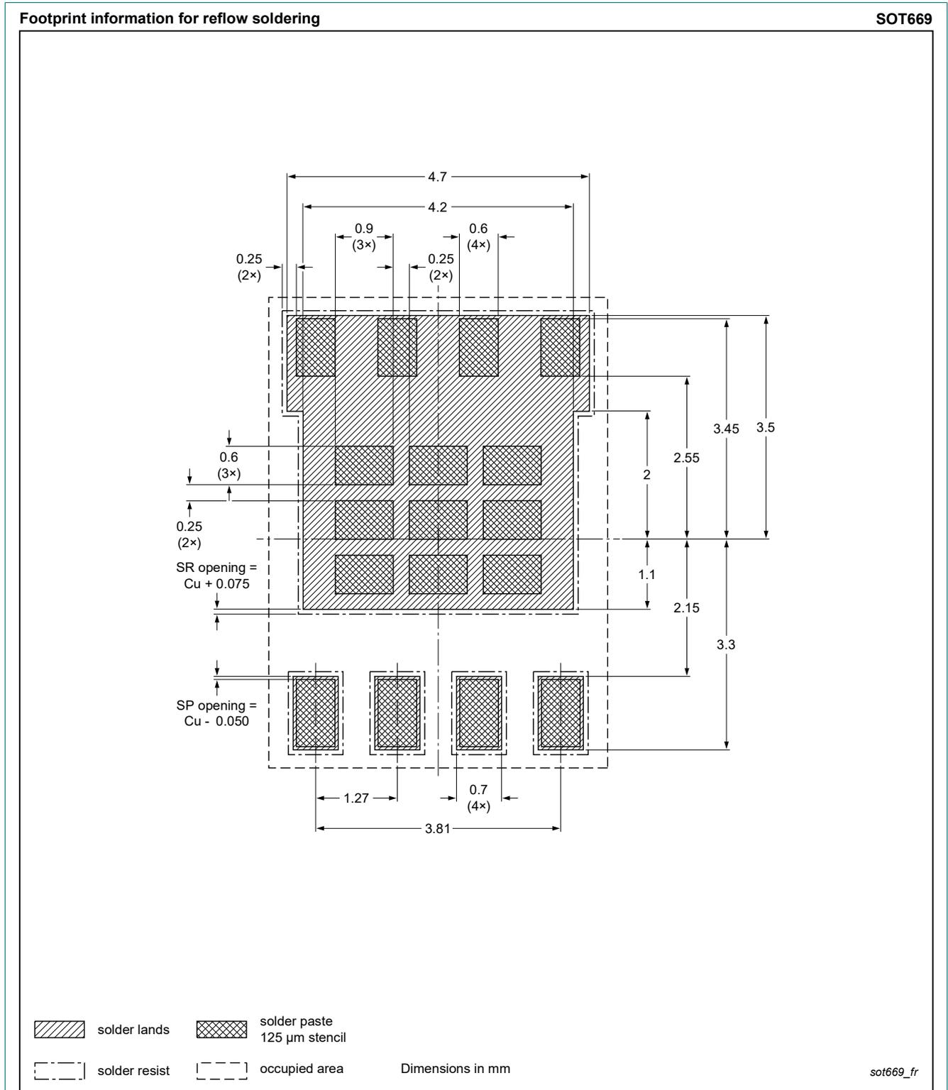
Fig. 18. Reflow soldering footprint for LFPAK56; Power-SO8 (SOT669)
