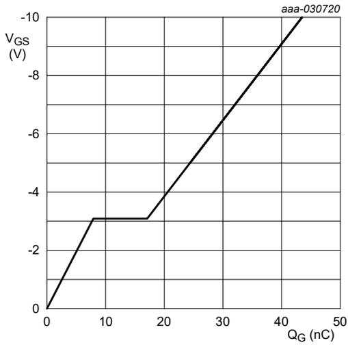
$V_{DS} = -30\text{ V}; I_D = -10.8\text{ A}; T_j = 25\text{ }^\circ\text{C}$
