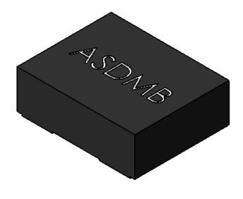
Note: Recommended using an approximately 0.01 uf bypass capacitor between PIN 2 and 4.
