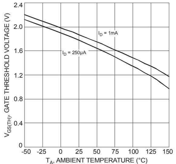
Fig. 6 Gate Threshold Variation vs. Ambient Temperature
