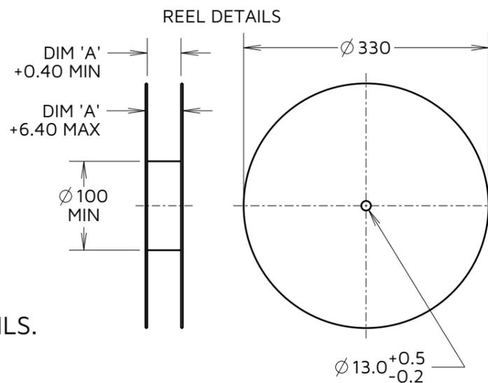
TAPE & REEL DETAILS ONLY. SEE SHEET 3 FOR CONNECTOR AND PCB LAYOUT DETAILS.
