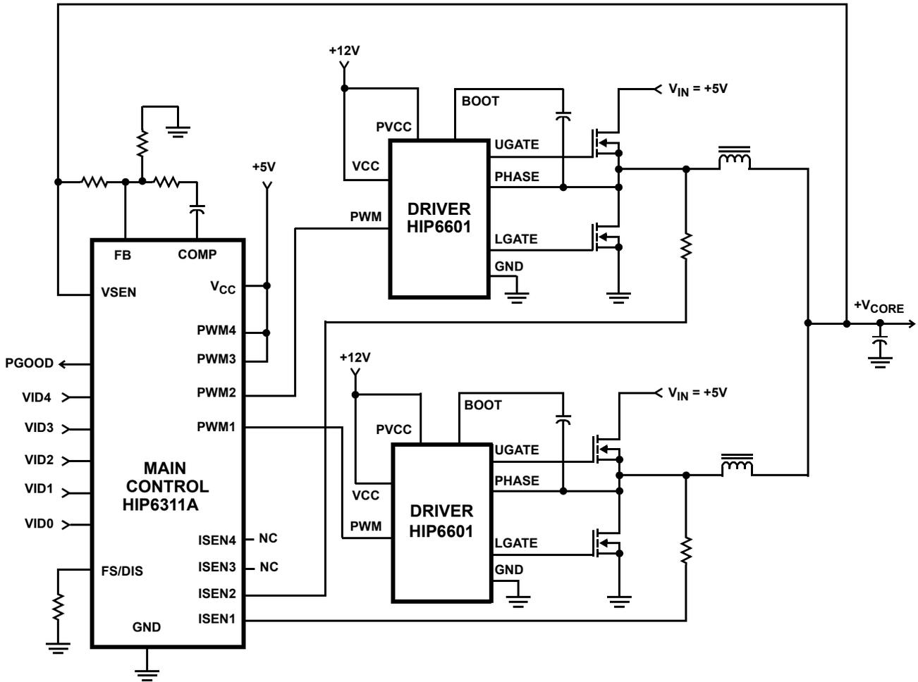
**Typical Application - 4 Phase Converter Using HIP6602 Gate Drivers**
