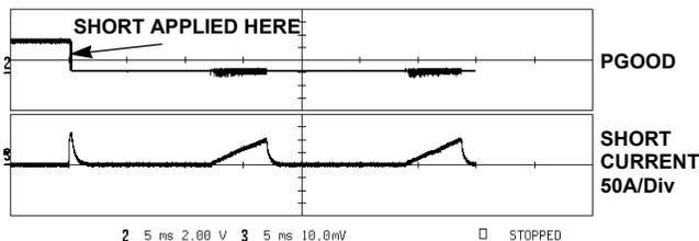
HICUP MODE. SUPPLY POWERED BY ATX SUPPLY
