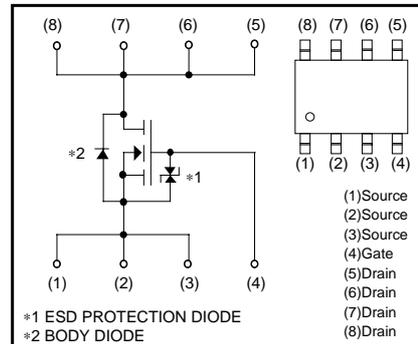
\*A protection diode is included between the gate and the source terminals to protect the diode against static electricity when the product is in use. Use the protection circuit when the fixed voltages are exceeded.
