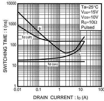
Fig.2 Switching Characteristics
