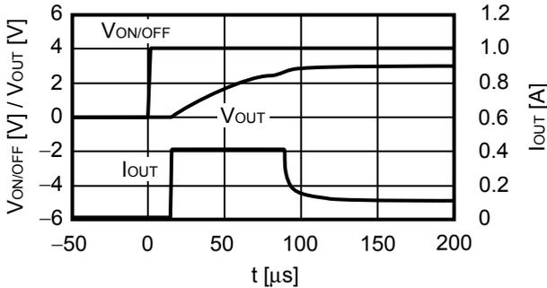
$V_{IN} = 4.0\text{ V}$ ,  $C_{OUT} = 4.7\ \mu\text{F}$ ,  $C_{IN} = 4.7\ \mu\text{F}$ ,  $I_{OUT} = 500\text{ mA}$
