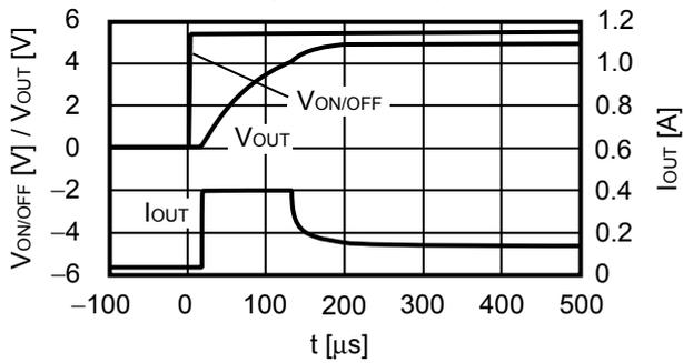
$V_{IN} = 5.5\text{ V}$ ,  $C_{OUT} = 4.7\ \mu\text{F}$ ,  $C_{IN} = 4.7\ \mu\text{F}$ ,  $I_{OUT} = 500\text{ mA}$
