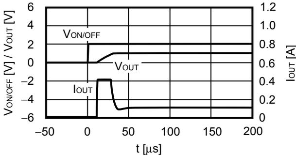
$V_{IN} = 2.0\text{ V}$ ,  $C_{OUT} = 4.7\ \mu\text{F}$ ,  $C_{IN} = 4.7\ \mu\text{F}$ ,  $I_{OUT} = 500\text{ mA}$
