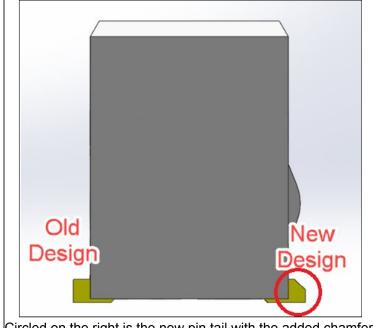
Circled on the right is the new pin tail with the added chamfer.
