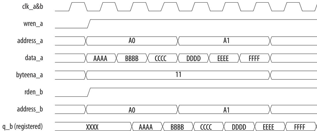
**Figure 2-4: Mixed-Port Read-During-Write: Old Data Mode**
