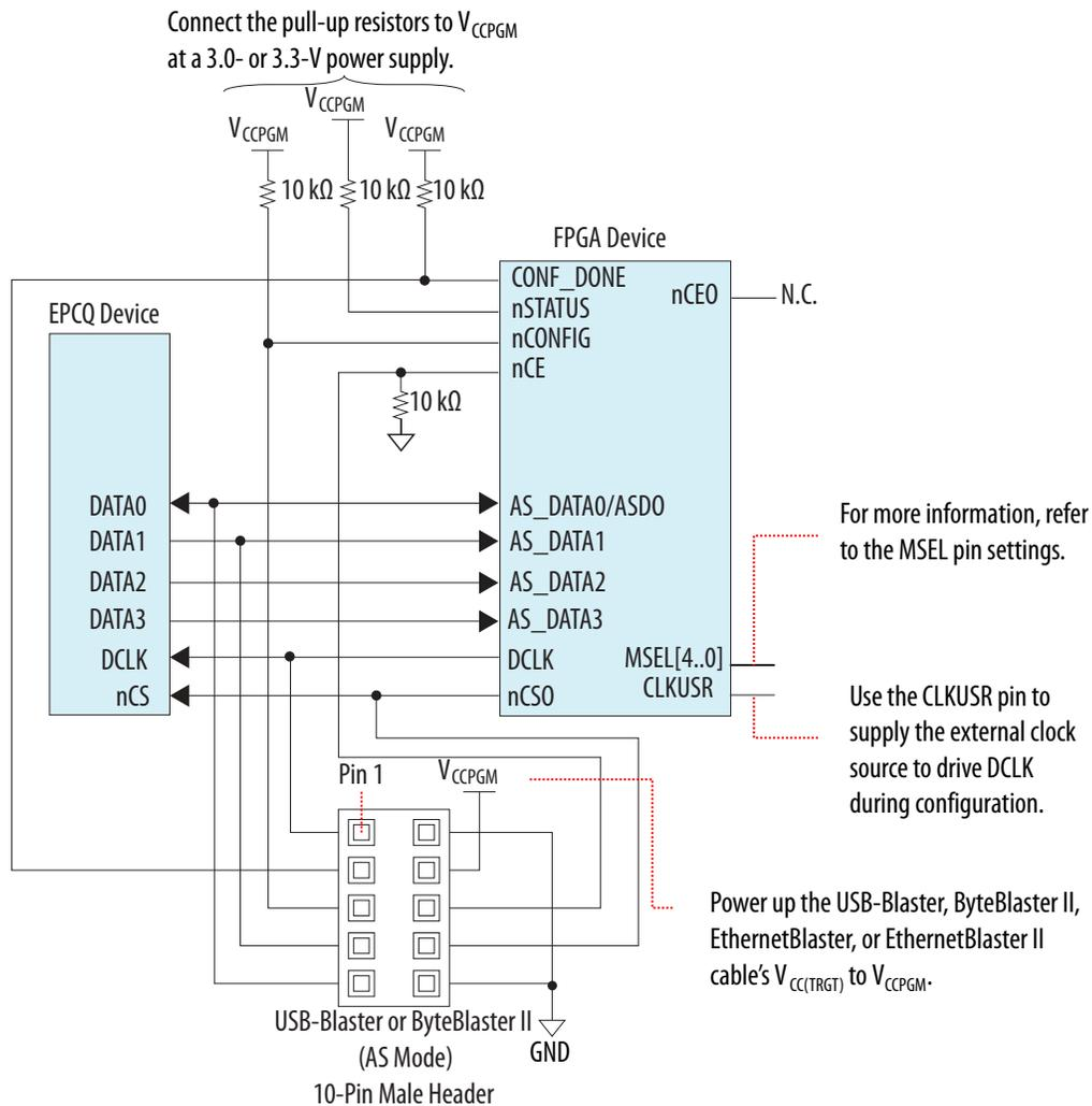
When programming the EPCS and EPCQ devices, the download cable disables access to the AS interface by driving the `nCE` pin high. The `nCONFIG` line is also pulled low to hold the Arria V device in the reset stage. After programming completes, the download cable releases `nCE` and `nCONFIG`, allowing the pull-down and pull-up resistors to drive the pin to GND and  $V_{CCPGM}$ , respectively.
