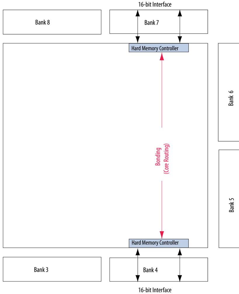
**Figure 7-27: Hard Memory Controllers Bonding Support in Arria V GX A5, A7, B1, B3, B5, and B7 Devices, and Arria V GT D3 and D7 Devices**
