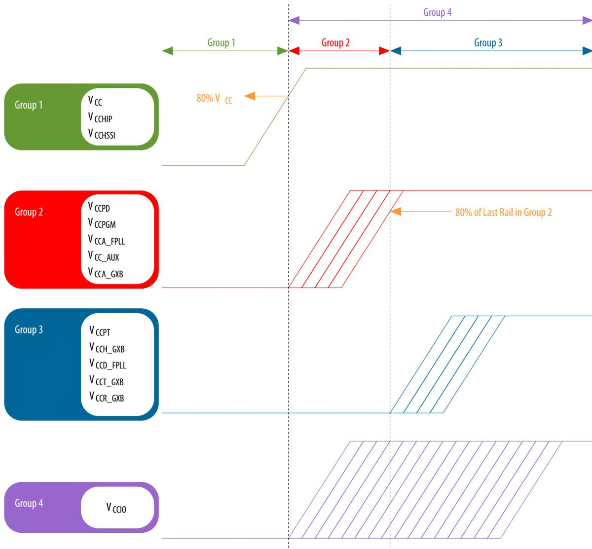
Arria V GZ devices may power down all power rails simultaneously. However, all rails must reach 0 V within 100 ms from the start of power-down.
