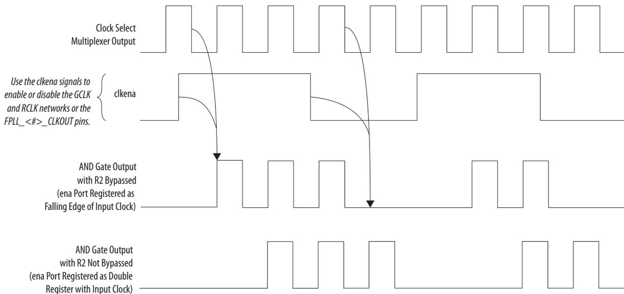
Arria V devices have an additional metastability register that aids in asynchronous enable and disable of the GCLK and RCLK networks. You can optionally bypass this register in the Intel Quartus Prime software.
