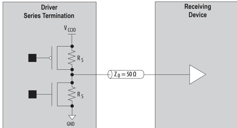
**R<sub>S</sub> OCT with Calibration in Arria V Devices**
