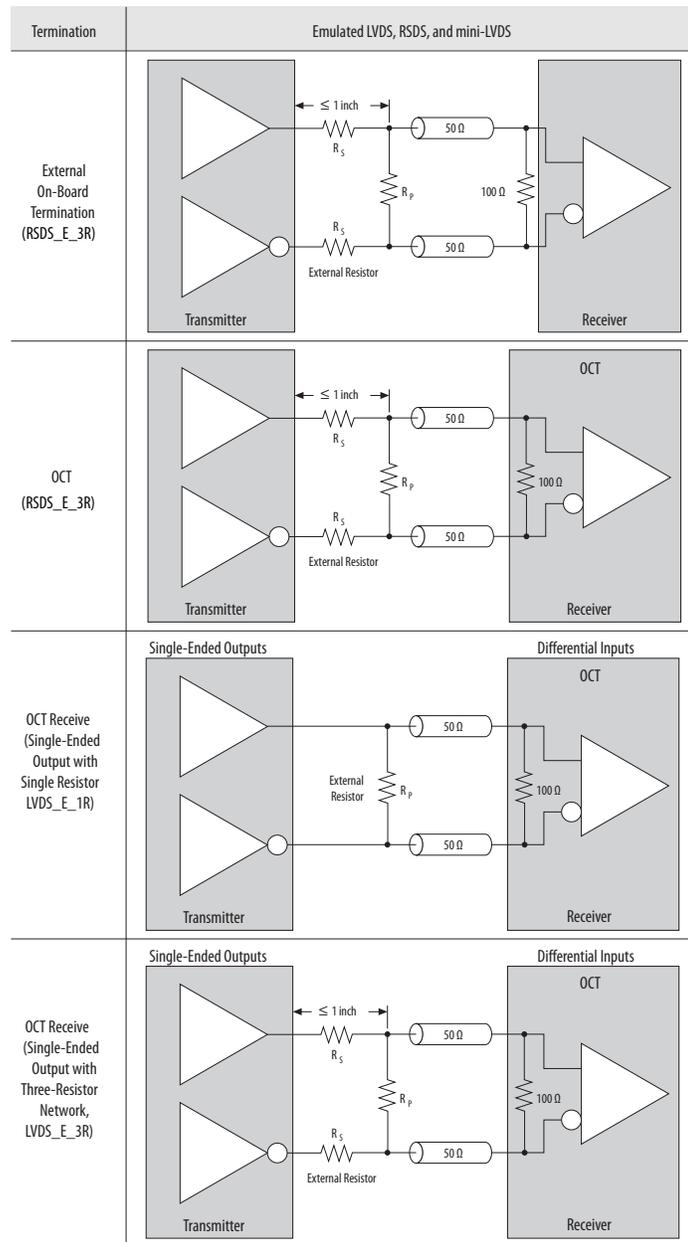
To meet the RSDS or mini-LVDS specifications, you require a resistor network to attenuate the output-voltage swing.
