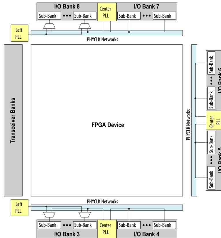
Figure 7-9: PHYCLK Networks in Arria V GX A5, A7, B1, B3, B5, and B7 Devices, and Arria V GZ E1, E3, E5, and E7 Devices
