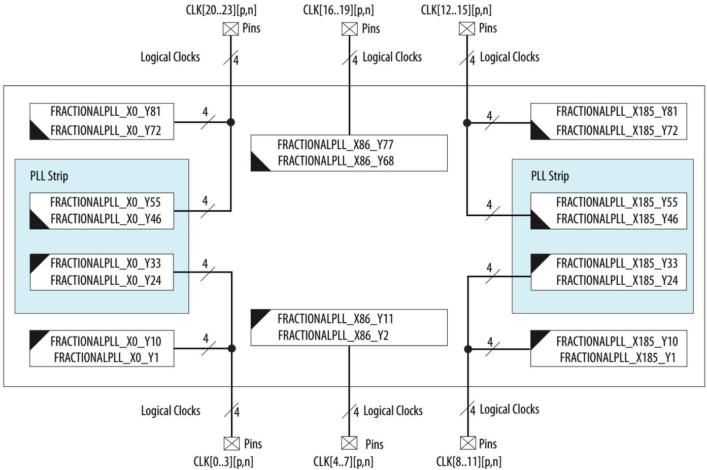
**Figure 4-19: PLL Locations for Arria V GZ E5 and E7 Devices**
