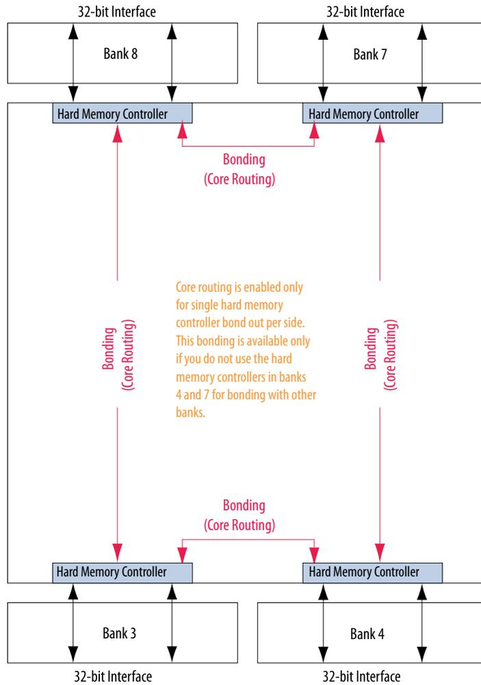
**Figure 7-28: Hard Memory Controllers in Arria V SX B3 and B5 Devices, and Arria V ST D3 and D5 Devices**
