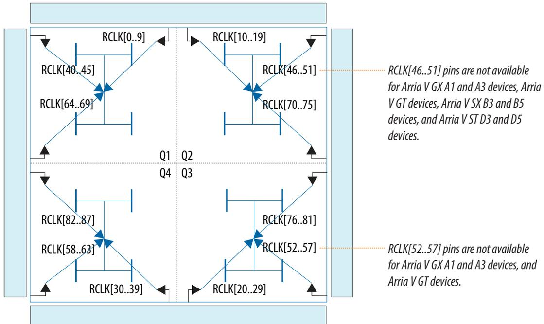
**Figure 4-3: RCLK Networks in Arria V GZ Devices**
