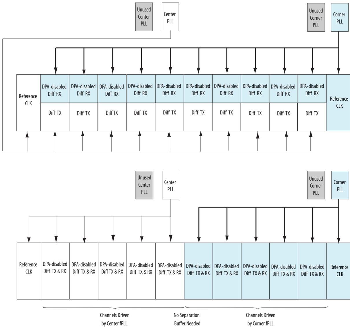
**Figure 6-18: Invalid Placement of DPA-disabled Differential I/Os Due to Interleaving of Channels Driven by the Corner and Center PLLs**
