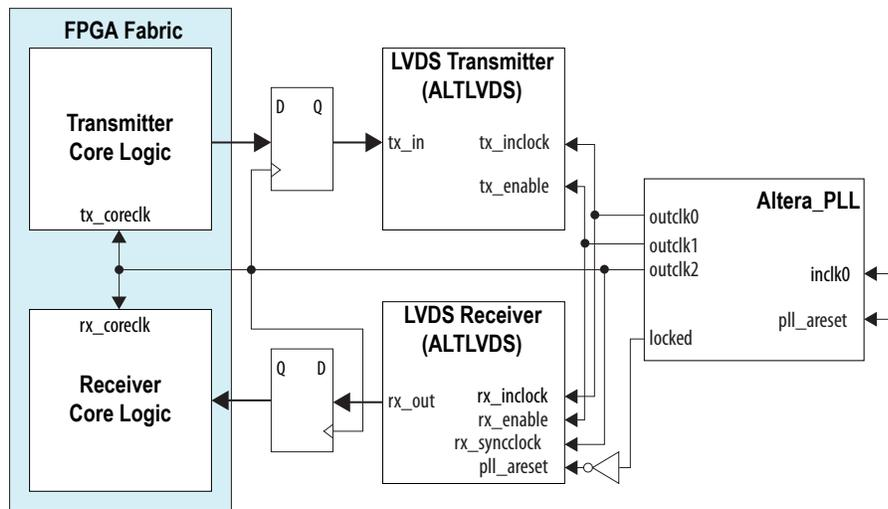
**Figure 6-9: LVDS Interface with the Altera\_PLL IP Core (With DPA)**
