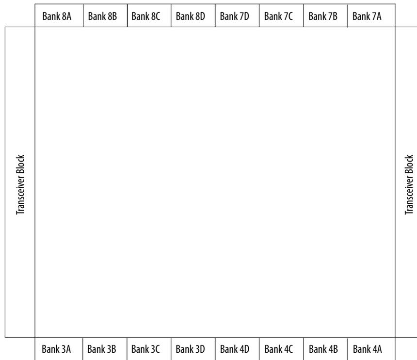
**Figure 5-4: I/O Banks for Arria V SX B3 and B5 Devices, and Arria V ST D3 and D5 Devices**
