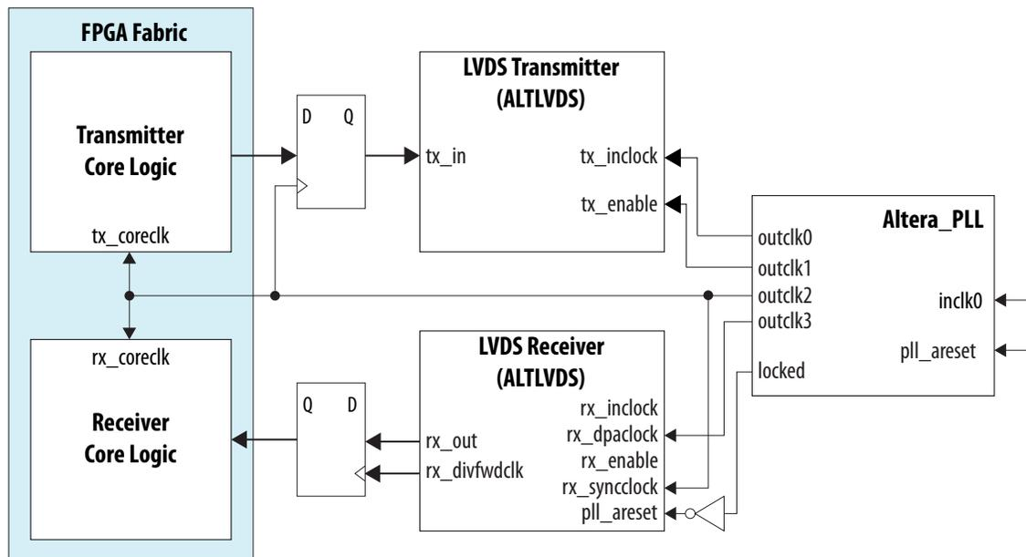
When generating the Altera\_PLL IP core, the **Left/Right PLL** option is configured to set up the PLL in LVDS mode. Instantiation of `pll_areset` is optional.
