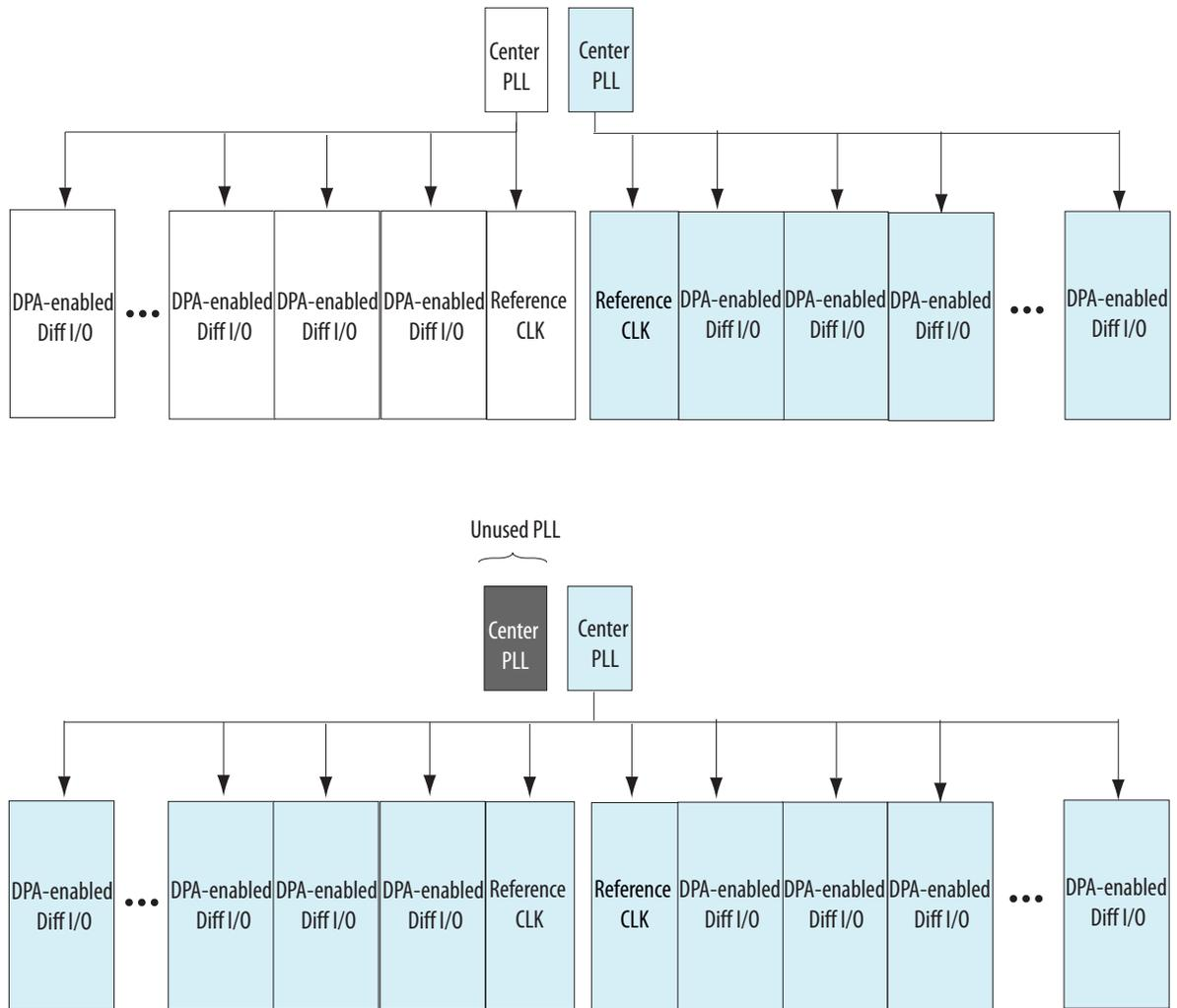
Figure 6-14: Center PLLs Driving DPA-enabled Differential I/Os in Arria V GZ Devices
