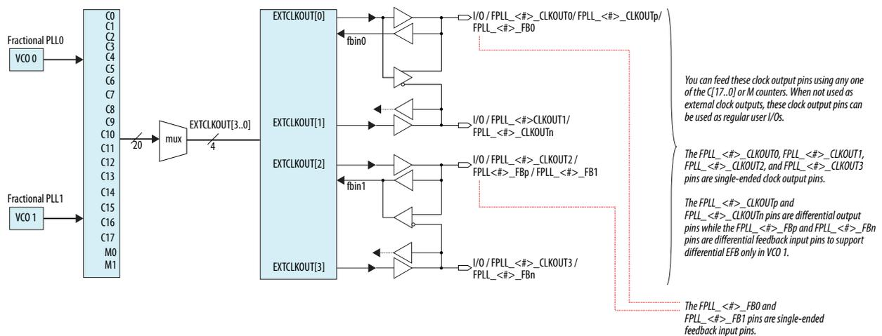
Each pin of a single-ended output pair can be either in-phase or 180° out-of-phase. To implement the 180° out-of-phase pin in a pin pair, the Intel Quartus Prime software places a NOT gate in the design into the IOE.
