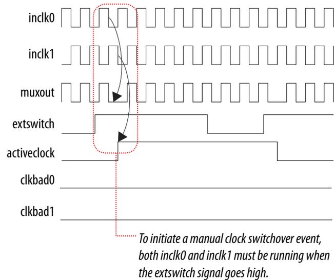
In automatic override with manual switchover mode, the `activeclock` signal mirrors the `extswitch` signal. Since both clocks are still functional during the manual switch, neither `clkbad` signal goes high. Because the switchover circuit is positive-edge sensitive, the falling edge of the `extswitch` signal does not cause the circuit to switch back from `inclk1` to `inclk0`. When the `extswitch` signal goes high again, the process repeats.
