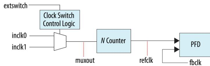
You can delay the clock switchover action by specifying the switchover delay in the ALTERA\_PLL IP core. When you specify the switchover delay, the `extswitch` signal must be held high for at least three `inclk` cycles plus the number of the delay cycles that has been specified to initiate a clock switchover.
