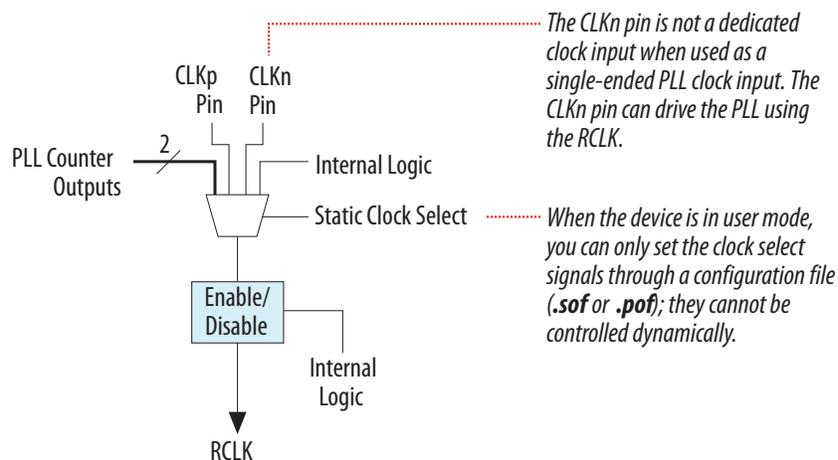
You can set the input clock sources and the `clkena` signals for the GCLK and RCLK network multiplexers through the Intel Quartus Prime software using the ALTCLKCTRL IP core.
