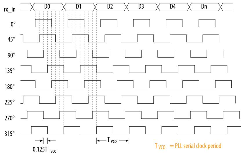
The DPA block continuously monitors the phase of the incoming serial data and selects a new clock phase if it is required. You can prevent the DPA from selecting a new clock phase by asserting the optional `RX_DPLL_HOLD` port, which is available for each channel.
