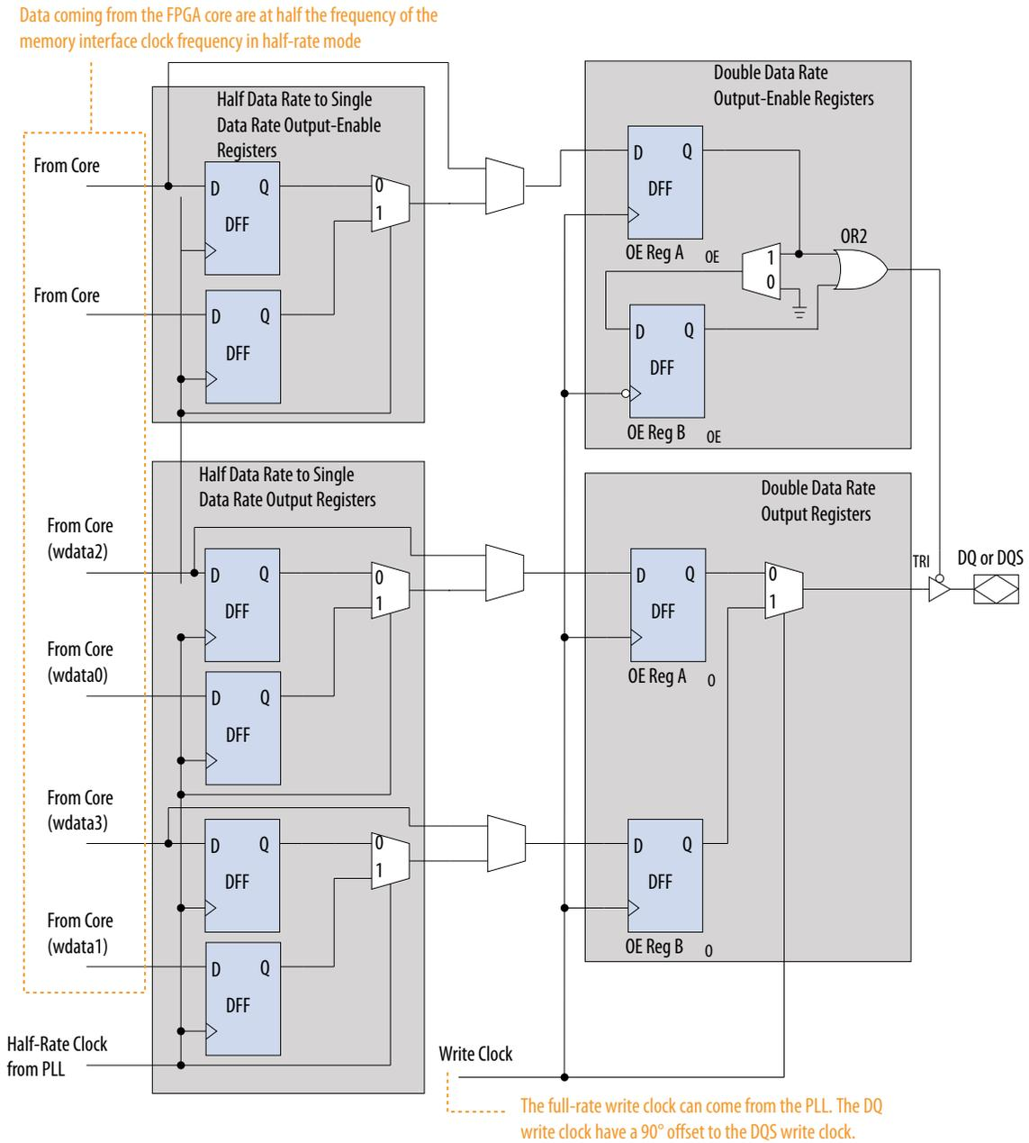
**Figure 7-20: IOE Output and Output-Enable Path Registers for Arria V GZ Devices**
