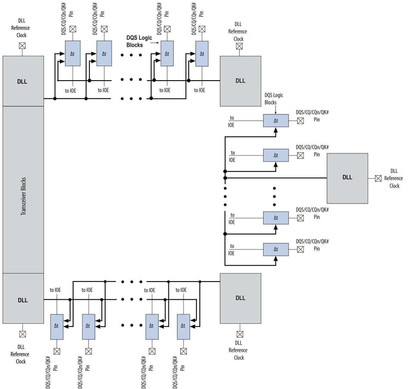
Figure 7-4: DQS/CQ/CQn/QK# Pins and DLLs in Arria V GX (A5, A7, B1, B3, B5, and B7), GT, and GZ Devices
