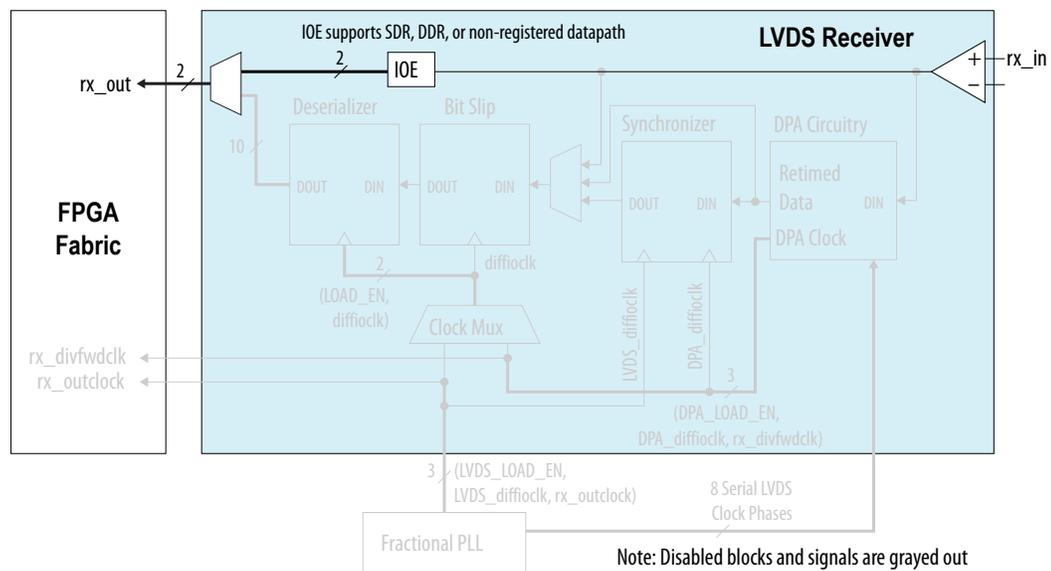
The IOE contains two data input registers that can operate in DDR or SDR mode. In DDR mode, `rx_inclock` clocks the IOE register. In SDR mode, data is directly passed through the IOE. In SDR and DDR modes, the data width from the IOE is 1 and 2 bits, respectively.
