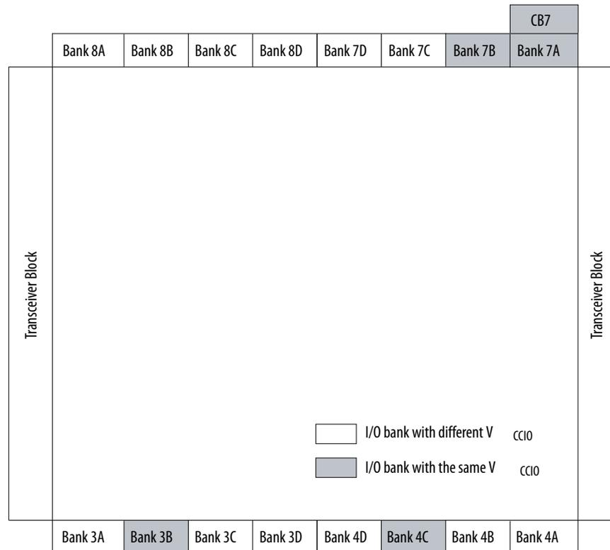
Because banks 3B, 4C, and 7B have the same  $V_{CCIO}$  as bank 7A, you can calibrate all four I/O banks (3B, 4C, 7A, and 7B) with the OCT calibration block (CB7) located in bank 7A.
