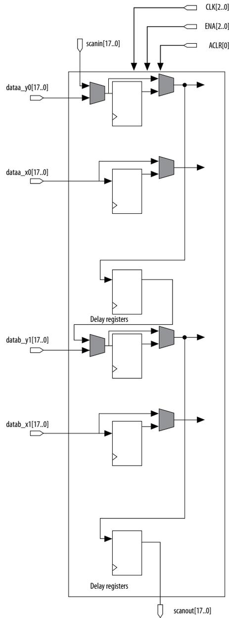
**Figure 3-8: Input Register of a Variable Precision DSP Block in 27 x 27 Mode for Arria V GZ Devices**
