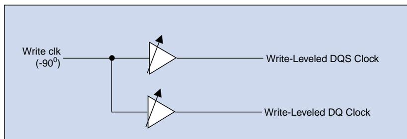
The -90° write clock of the UniPHY IP feeds the write-leveling circuitry to produce the clock to generate the DQS and DQ signals. During initialization, the UniPHY IP picks the correct write-leveled clock for the
