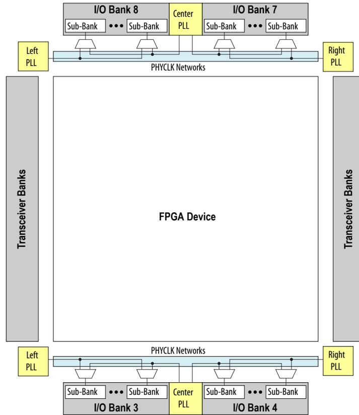
Figure 7-10: Arria V PHYCLK Networks in Arria V SX B3 and B5 Devices, and Arria V ST D3 and D5 Devices
