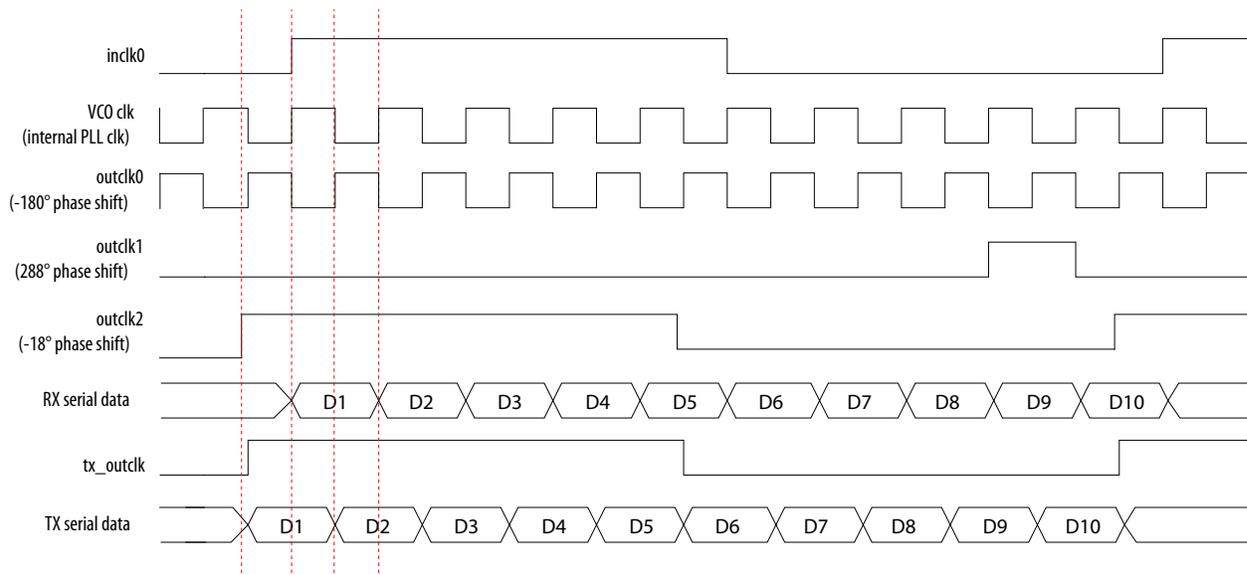
Table 6-8: Example: Generating Output Clocks Using an Altera\_PLL IP Core (With DPA and Soft-CDR Mode)
