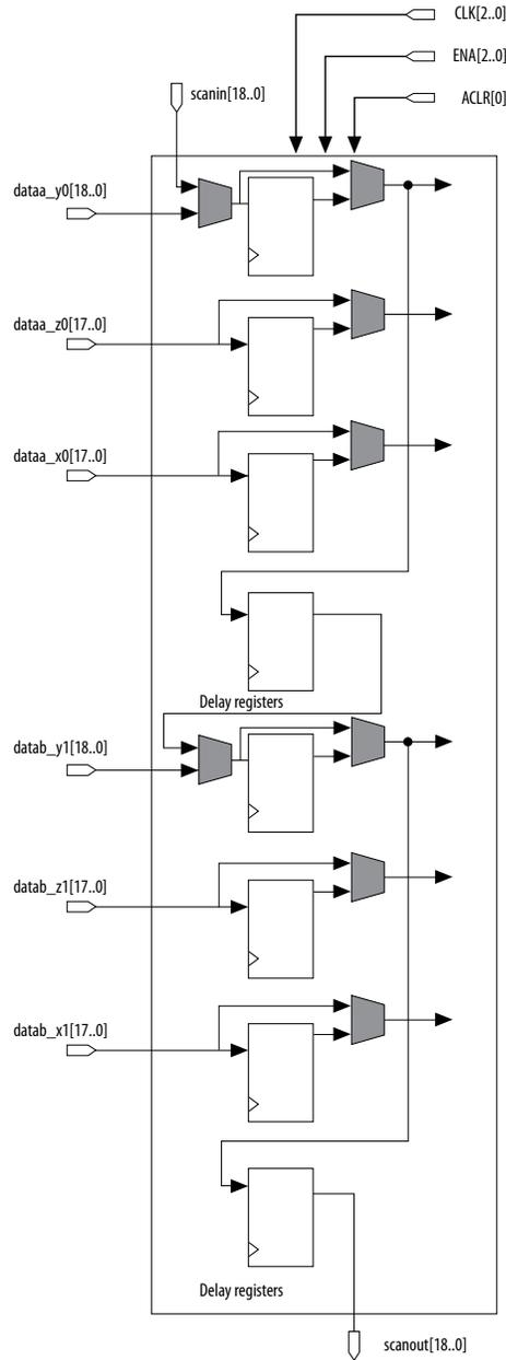
**Figure 3-6: Input Register of a Variable Precision DSP Block in 27 x 27 Mode for Arria V GX, GT, SX, and ST Devices**
