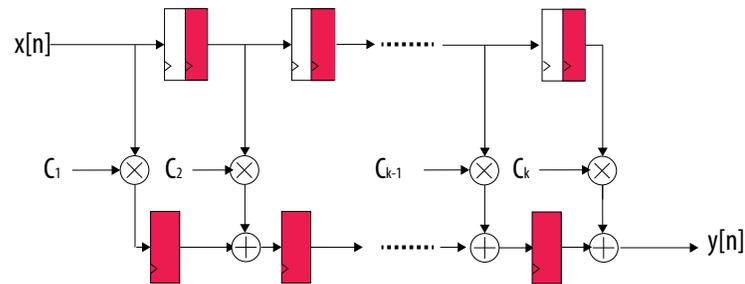
Arria V variable precision DSP blocks support the following systolic FIR structures:
