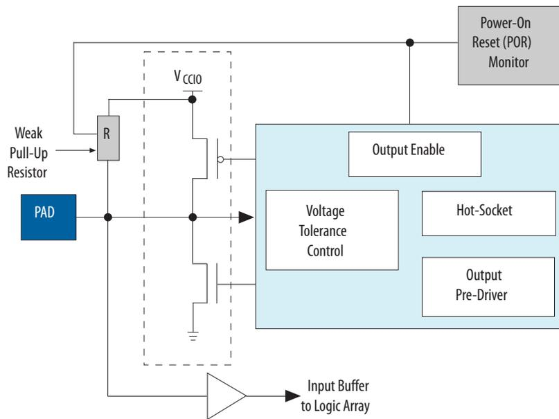
The POR circuitry monitors the voltage level of the power supplies and keeps the I/O pins tri-stated until the device is in user mode. The weak pull-up resistor (R) in the Arria V input/output element (IOE) is enabled during configuration download to keep the I/O pins from floating.
