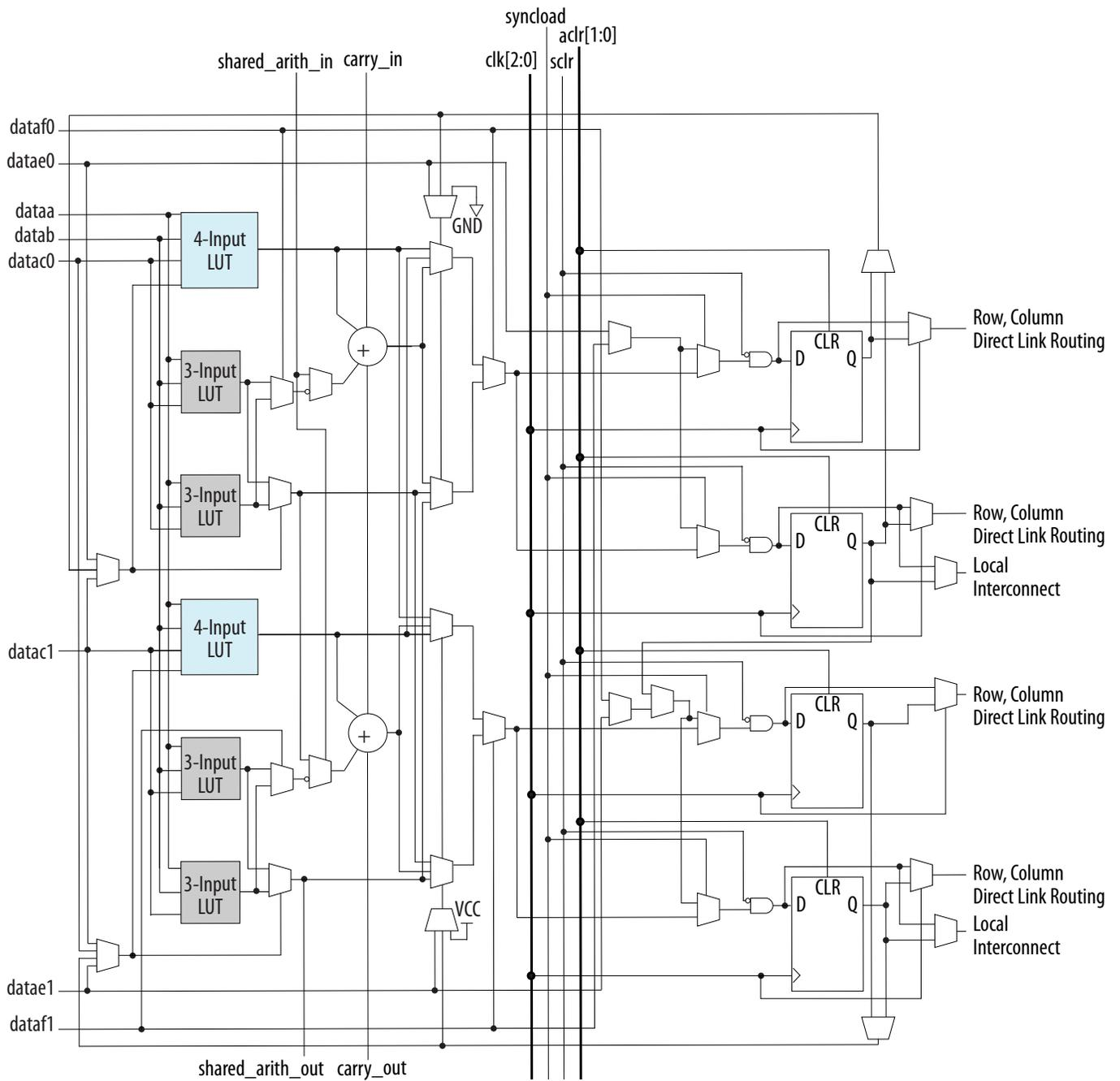
Figure 1-10: ALM Connection Details for Arria V GZ Devices
