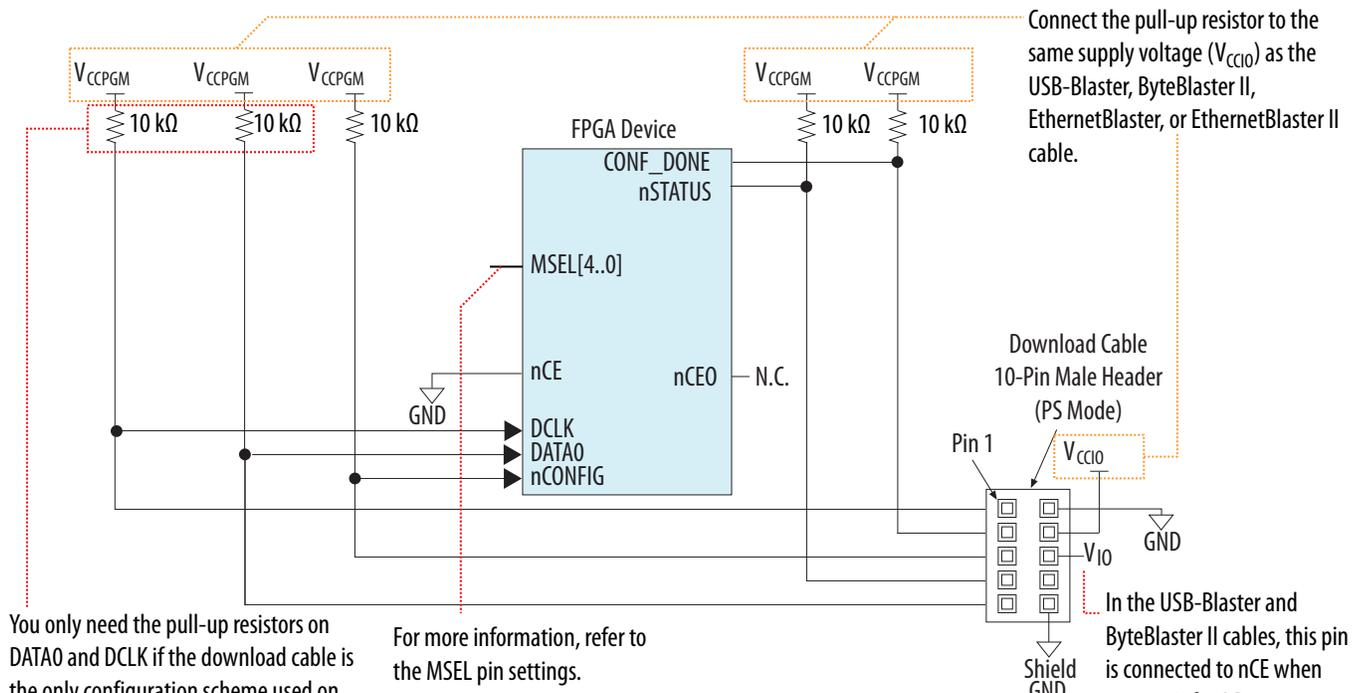
Connect the pull-up resistor to the same supply voltage ( $V_{CCIO}$ ) as the USB-Blaster, ByteBlaster II, EthernetBlaster, or EthernetBlaster II cable.
