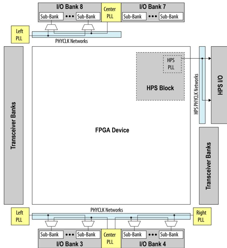
The PHYCLK network can be used to drive I/O sub-banks in each I/O bank. Each I/O sub-bank can be driven by only one PHYCLK network—all I/O pins in an I/O sub-bank are driven by the same PHYCLK network.
