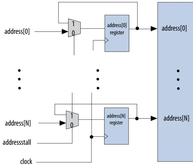
**Figure 2-8: Address Clock Enable During Read Cycle**
