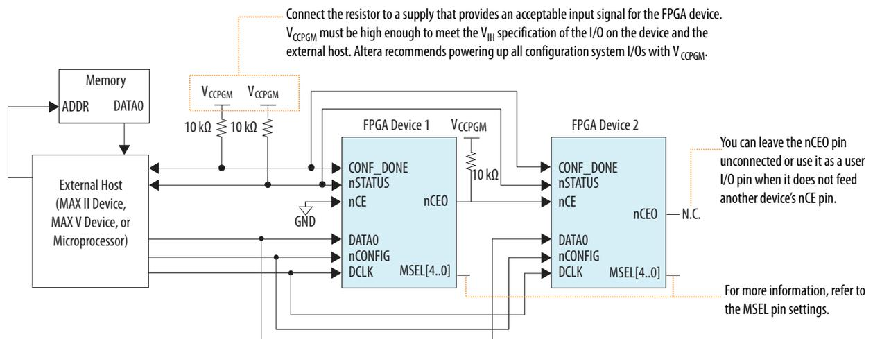
After a device completes configuration, its nCEO pin is released low to activate the nCE pin of the next device in the chain. Configuration automatically begins for the second device in one clock cycle.
