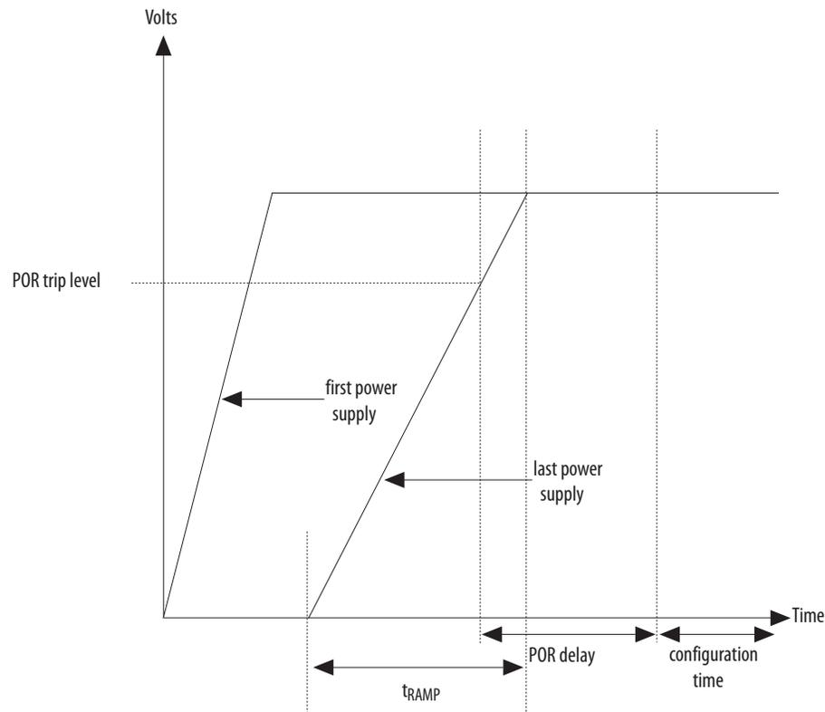
The Arria V POR circuitry uses an individual detecting circuitry to monitor each of the configuration-related power supplies independently. The main POR circuitry is gated by the outputs of all the individual detectors. The main POR signal is asserted when the power starts to ramp up. This signal is released after the last ramp-up power reaches the POR trip level during power up.
