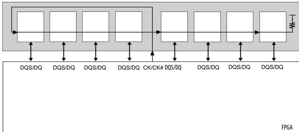
Because the data and read strobe signals are still point-to-point, take special care to ensure that the timing relationship between the CK/CK# and DQS signals ( $t_{DQSS}$ ,  $t_{DSS}$ , and  $t_{DSH}$ ) during a write is met at every device on the modules. In a similar way, read data coming back into the FPGA from the memory is also staggered.
