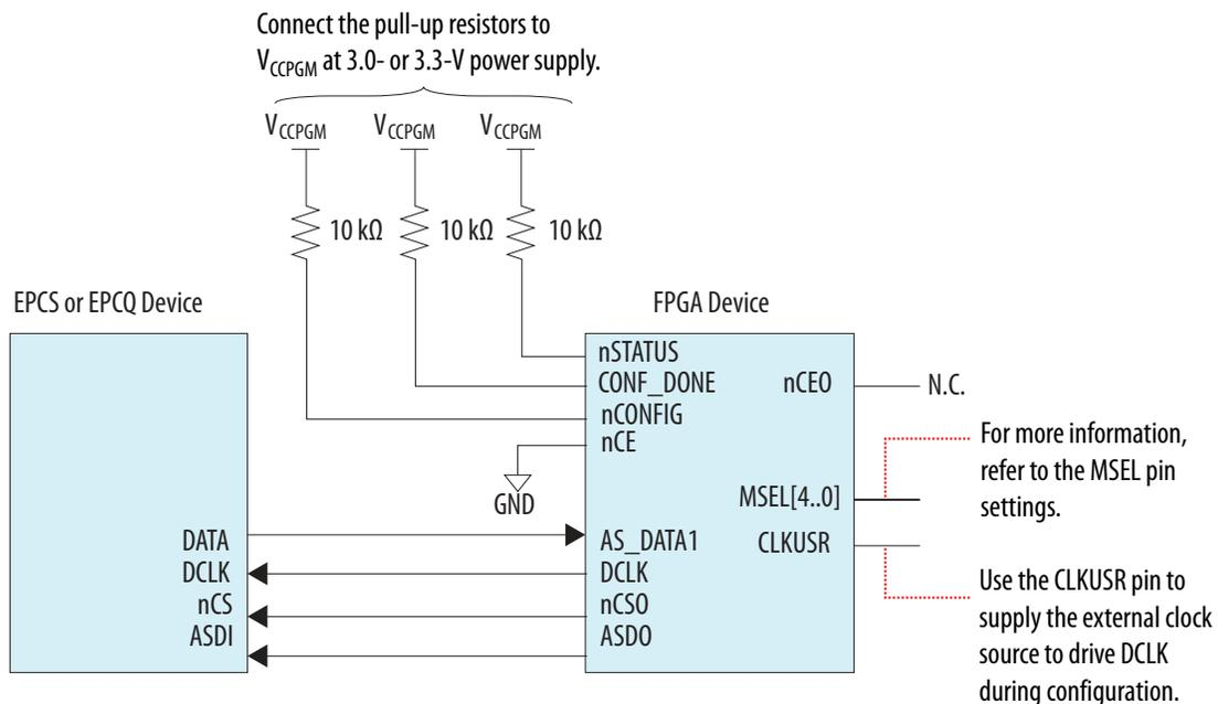
Figure 8-10: Single Device AS x4 Mode Configuration
