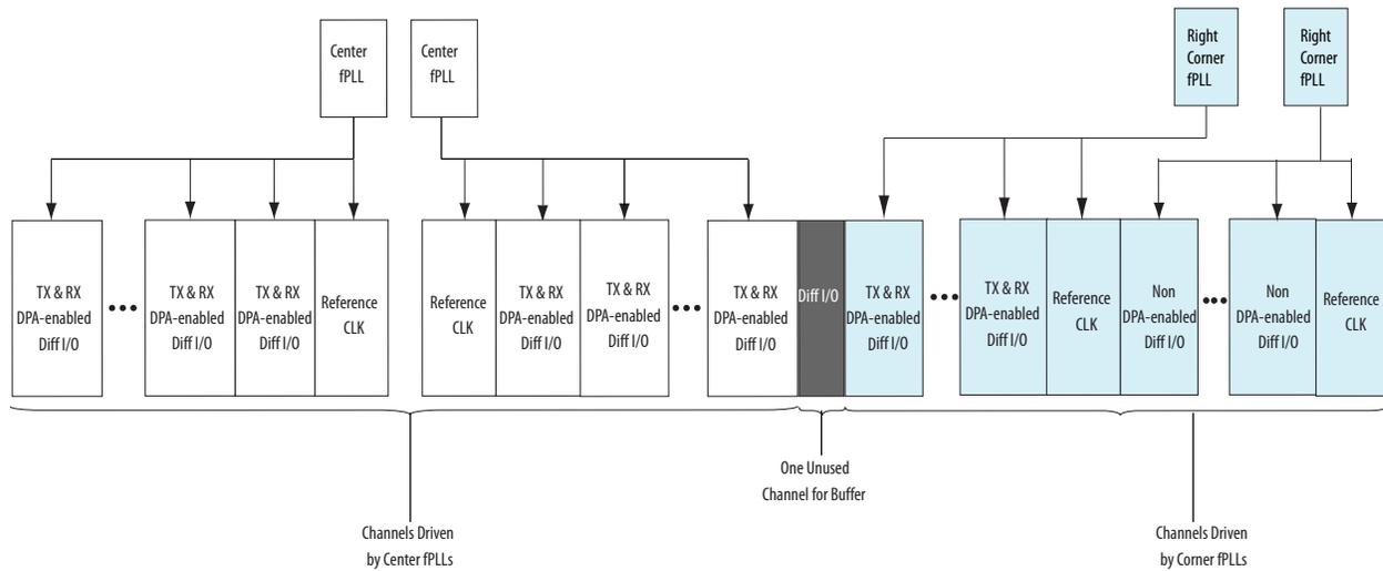
This separation prevents noise mixing because the two groups can operate at independent frequencies. No separation is necessary if a single PLL is driving both the DPA-enabled channels and DPA-disabled channels.
