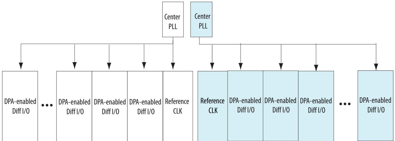
Figure 6-15: Invalid Placement of DPA-enabled Differential I/Os Driven by Both Center PLLs
