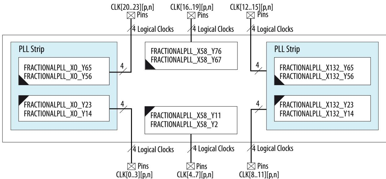
**Figure 4-16: PLL Locations for Arria V GX B1 and B3 Devices, and Arria V GT D3 Device**
