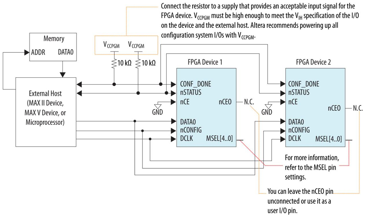
The nCE pins of the devices in the chain are connected to GND, allowing configuration for these devices to begin and end at the same time.
