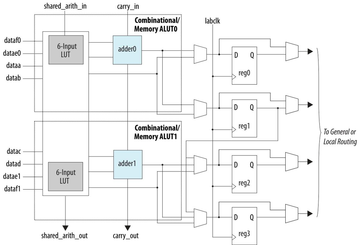
Figure 1-8: ALM High-Level Block Diagram for Arria V GZ Devices
