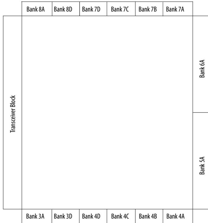
**Figure 5-3: I/O Banks for Arria V GX A5, A7, B1, B3, B5, and B7 Devices, Arria V GT C7, D3, and D7 Devices, and Arria V GZ Devices**
