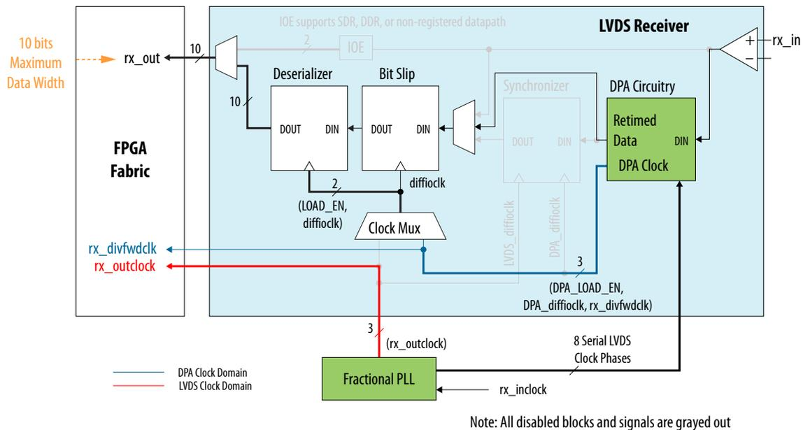
In soft-CDR mode, the synchronizer block is inactive. The DPA circuitry selects an optimal DPA clock phase to sample the data. Use the selected DPA clock for bit-slip operation and deserialization. The DPA block also forwards the selected DPA clock, divided by the deserialization factor called `rx_divfwdclk`, to the FPGA fabric, along with the deserialized data. This clock signal is put on the periphery clock (PCLK) network.
