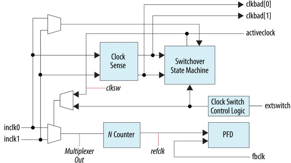
When the current reference clock is not present, the clock sense block automatically switches to the backup clock for PLL reference. You can select a clock source as the backup clock by connecting it to the `inclk1` port of the PLL in your design.
