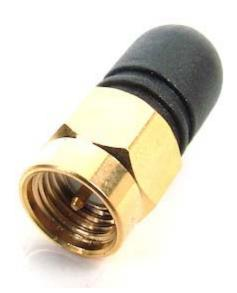
The Delta 19 is an extremely small 2.4GHz direct connect antenna only 19mm long including the connector. It is intended for small or hand held products that need WiFi, Zigbee or Bluetooth connectivity and where any other size stubby antenna would be too large. Very small modules and discrete monitoring devices will demand the Delta 19. The Delta 19 is available with standard SMA male connector or the normal WiFi SMA male RP connector.
