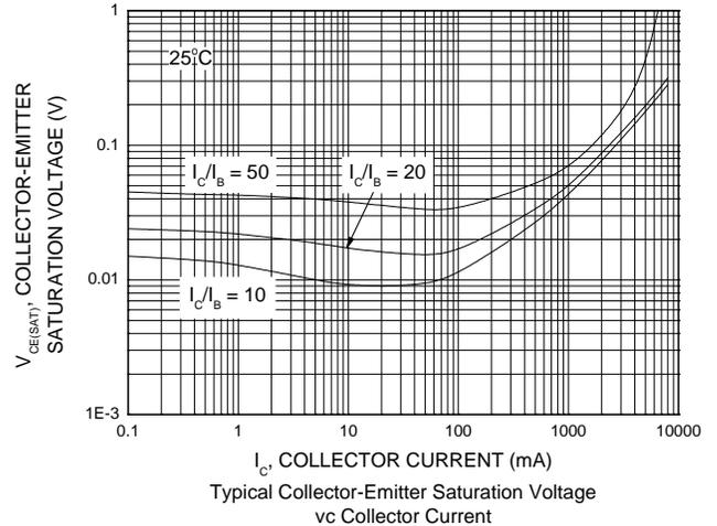
Typical Collector-Emitter Saturation Voltage vs Collector Current
