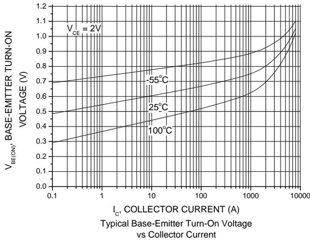
Typical Base-Emitter Turn-On Voltage vs Collector Current
