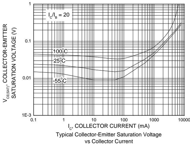
Typical Collector-Emitter Saturation Voltage vs Collector Current
