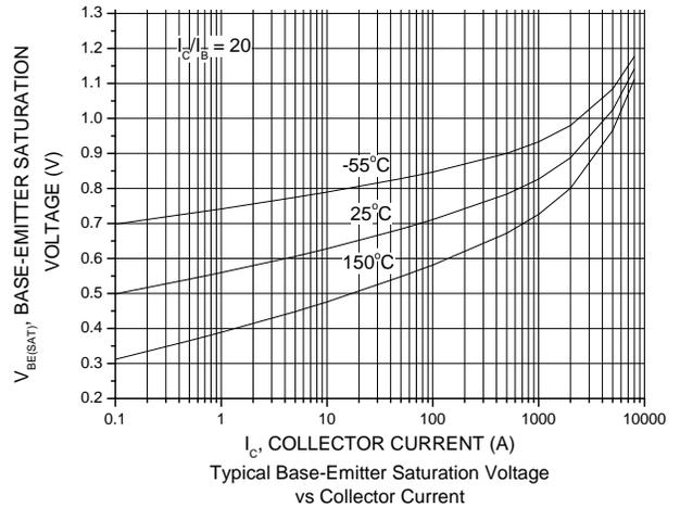
Typical Base-Emitter Saturation Voltage vs Collector Current
