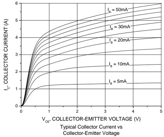
Typical Collector Current vs Collector-Emitter Voltage
