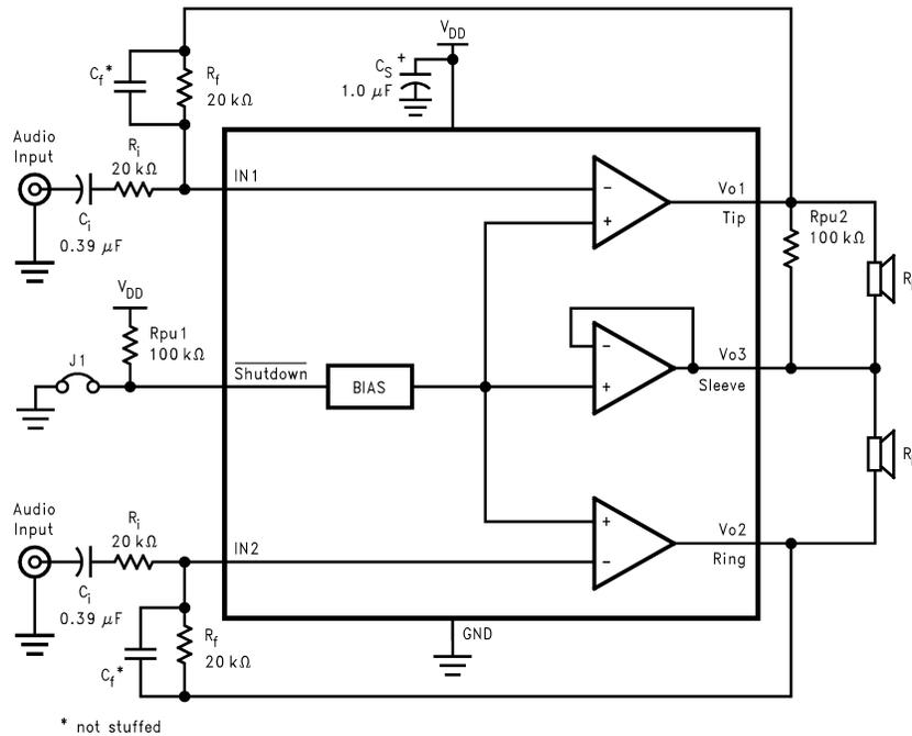
A. R<sub>PU2</sub> is not required. It is used for test measurement purposes only.
