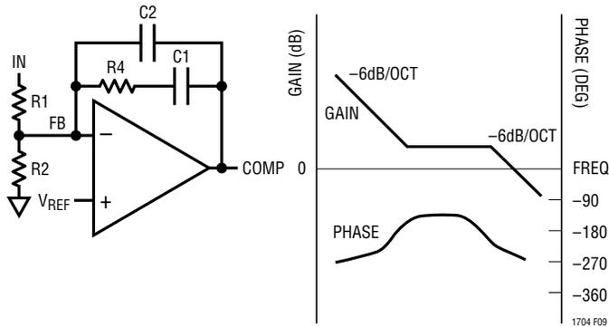
Figure 9. Type 2 Schematic and Transfer Function
