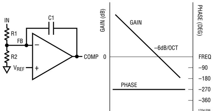
Figure 8. Type 1 Schematic and Transfer Function
