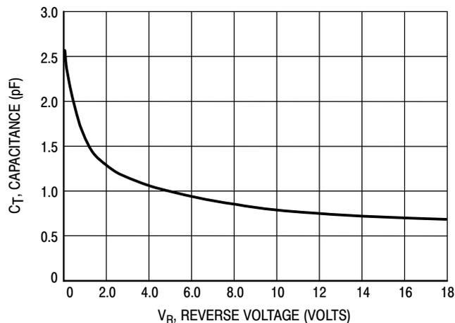
Figure 4. Typical Capacitance
