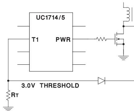
Figure 8. Using The Timer Input For Zero-Voltage Sensing
