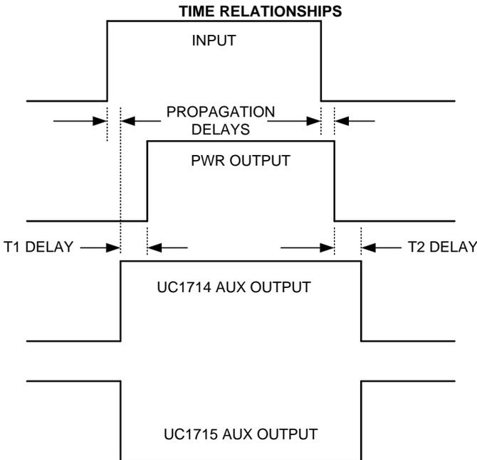
(2) T1 delay is defined from the 50% point of the transition edge of AUX to the 10% of the rising edge of PWR. T2 delay is defined from the 90% of the falling edge of PWR to the 50% point of the transition edge of AUX.
