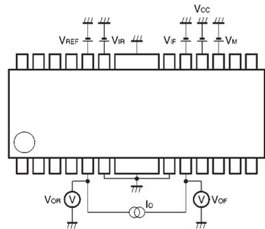
VCE is the sum of the high- and low-side output transistor C-E voltages. The direction of the Io current is from the HIGH level to the LOW level output pin.
