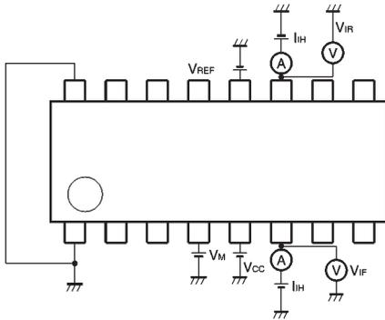
\* Refer to the truth table for output mode. HIGH and LOW level input voltages correspond to the readings of  $V_{if}$  and  $V_{ir}$  voltmeters, respectively. The HIGH level input current is represented by the  $I_{ih}$  ammeter reading when  $V_{in} = 2V$ .
