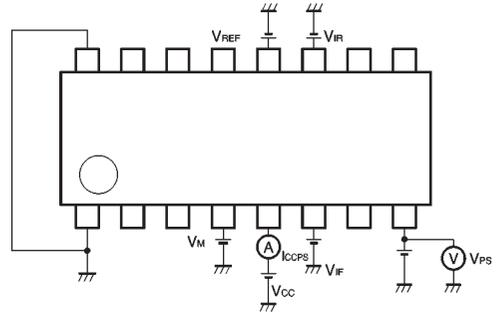
The power save mode ON voltage is represented by the  $V_{ps}$  reading when  $I_{ccps}$  is  $15\mu A$  or less. The power save mode OFF voltage is represented by the  $V_{ps}$  reading when  $I_{ccps}$  is more than  $15\mu A$ .
