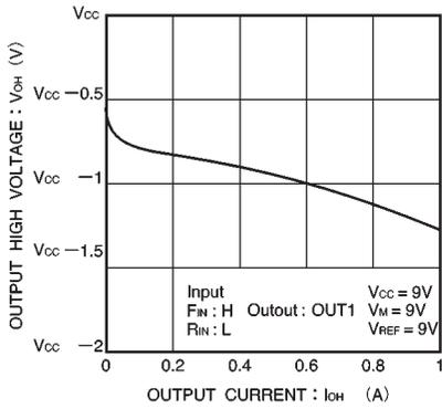
Fig.15 Output high level voltage vs. output current
