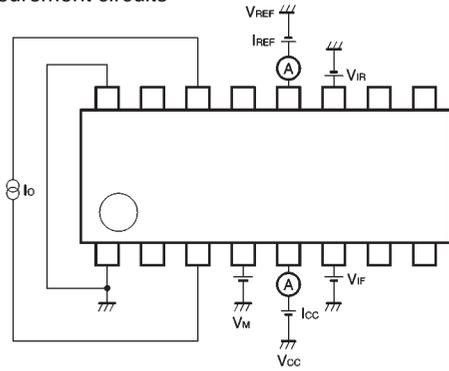
\* Refer to the truth table for output mode. The supply current is represented by the  $I_{cc}$ -value, and the  $V_{ref}$  sink current is represented by the  $I_{ref}$ -value. The direction of the  $I_o$  current is from the HIGH level to the LOW level output pin.
