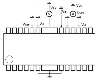
The power save mode ON voltage is represented by the VPS reading when ICCPS is 15 μA or less. The power save mode OFF voltage is represented by the VPS reading when ICCPS is more than 15 μA.
