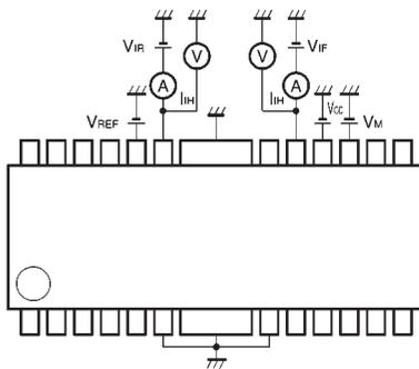
\* Refer to the truth table for output mode. HIGH and LOW level input voltages correspond to the readings of VIF and VIR voltmeters, respectively. The HIGH level input current is represented by the IIR ammeter reading when VIN = 2 V.
