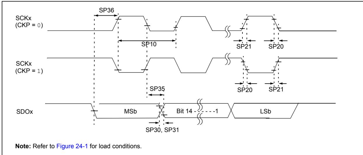
**TABLE 24-33: SPIx MASTER MODE (HALF-DUPLEX, TRANSMIT ONLY) TIMING REQUIREMENTS**
