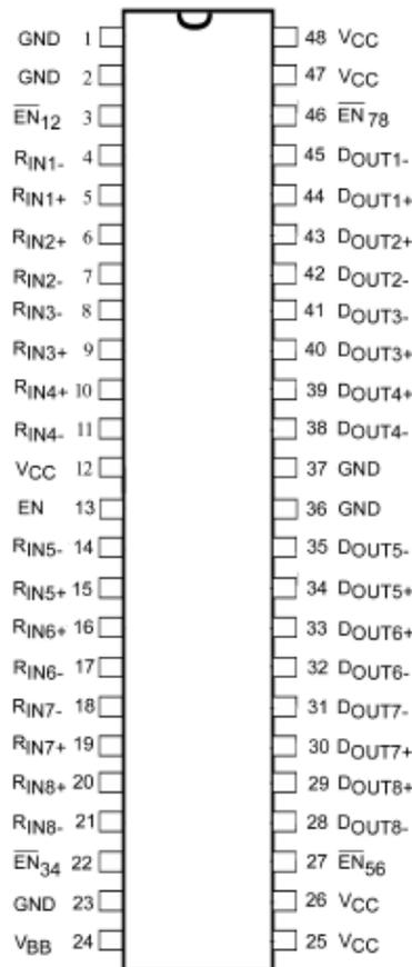
Figure 1. Pin Configuration
