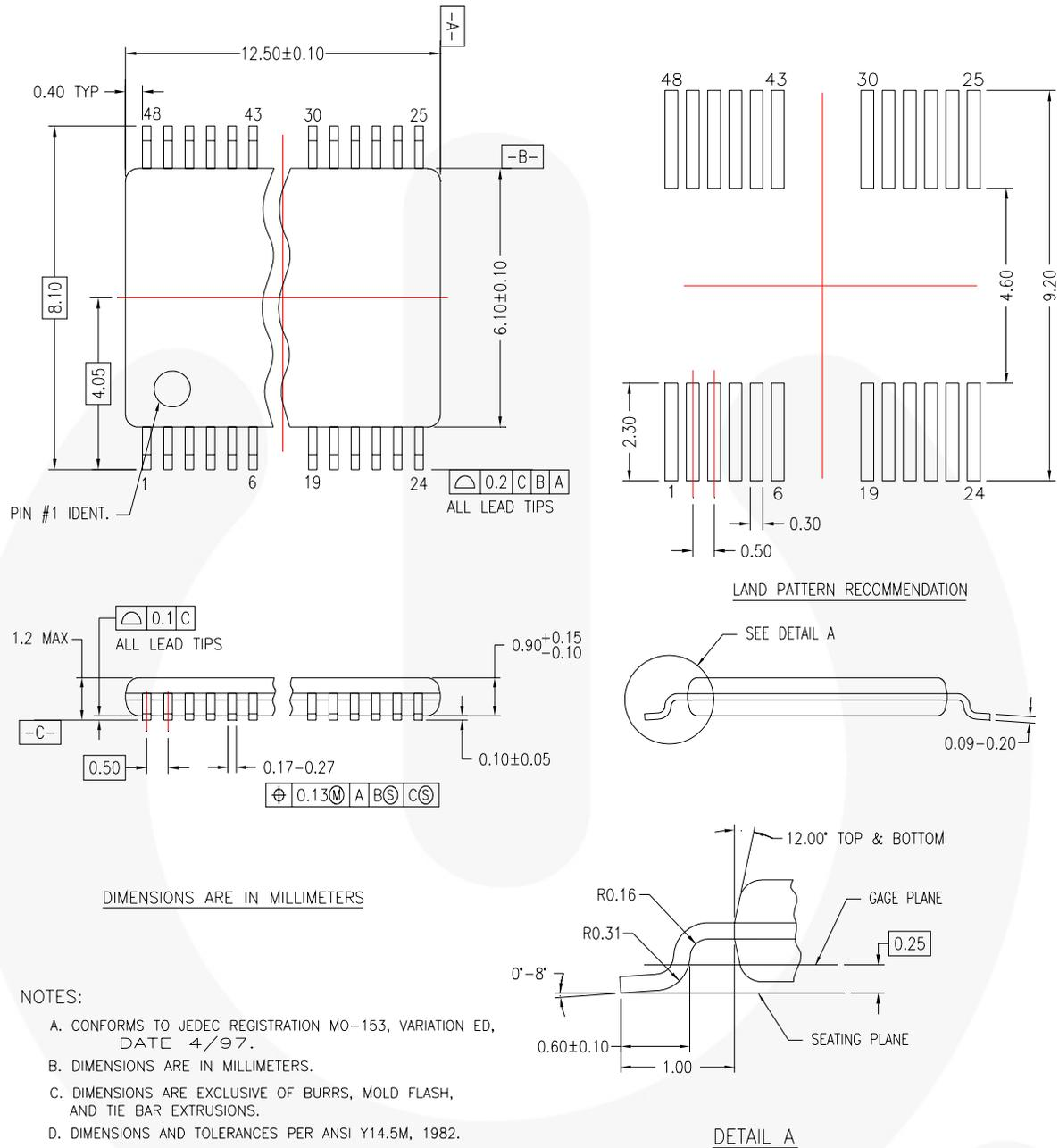
**Figure 9. 48-Lead, Thin Shrink Small Outline Package (TSSOP), JEDEC MO-153, 6.1mm Wide**
