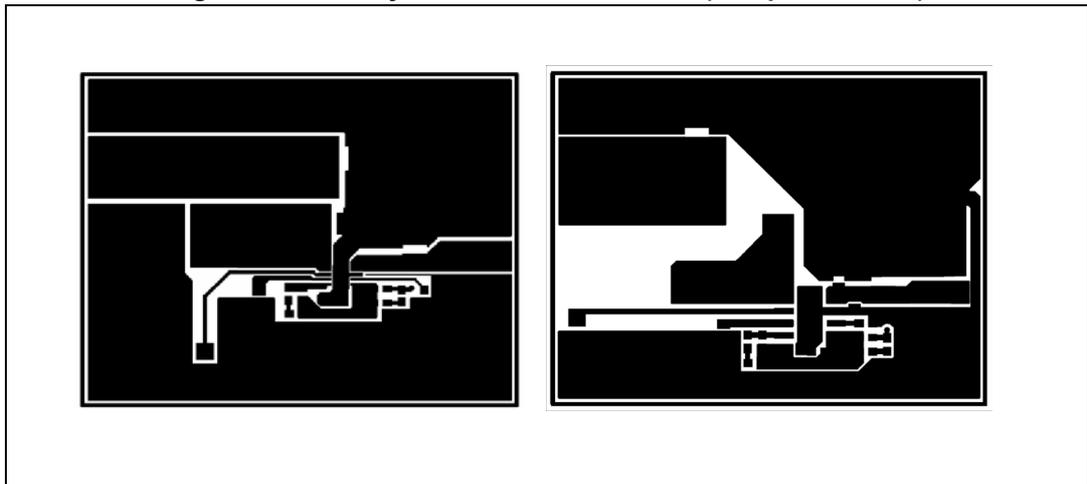
Figure 21. PCB layout: L5987 and L5987A (bottom side)
