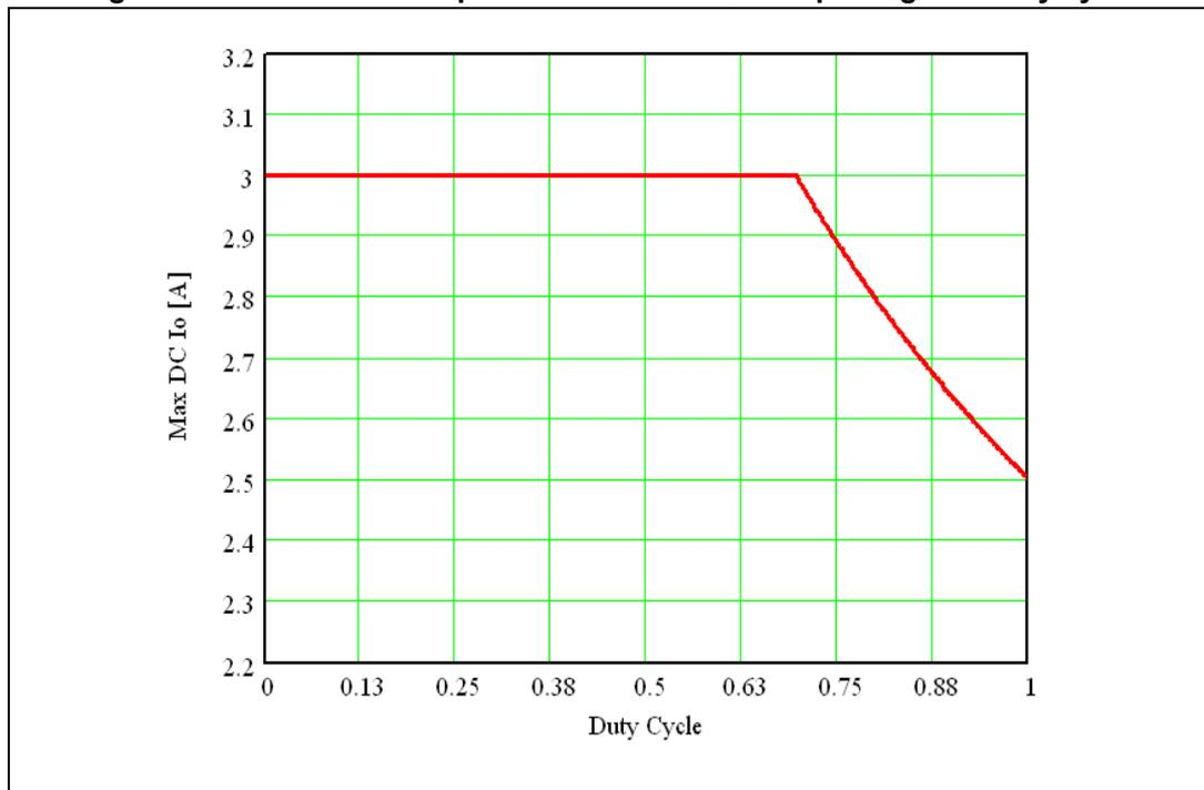
*Note:* For duty cycles lower than 69%, the RMS current does not limit the maximum DC output current of 3 A. For duty cycles higher than the 69% the maximum DC output current is limited by the RMS current (see [Equation 5](#)).
