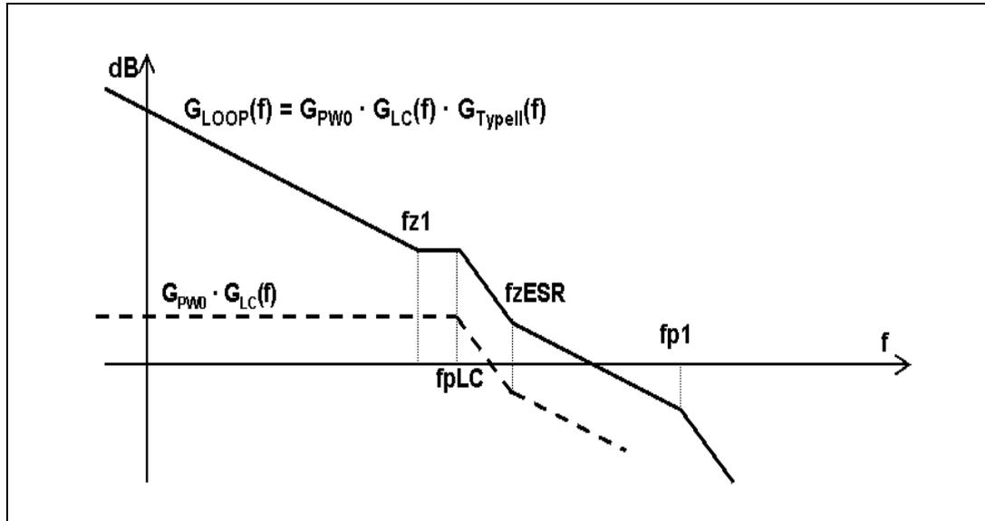
The guidelines for positioning the poles and the zeroes and for calculating the component values can be summarized as follows:
