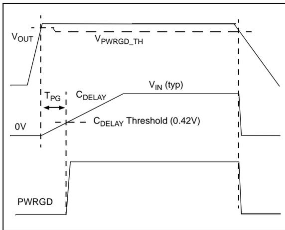
**FIGURE 4-4:** C<sub>DELAY</sub> and PWRGD Timing Diagram.
