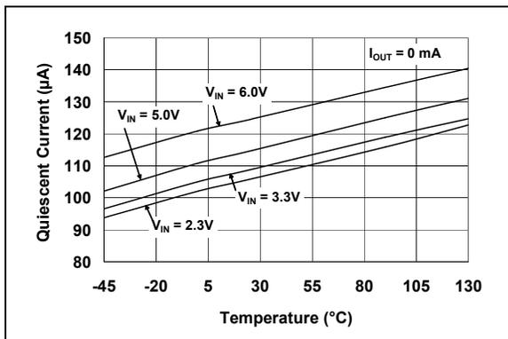
**FIGURE 2-3:** Quiescent Current vs. Junction Temperature (1.8V Adjustable).
