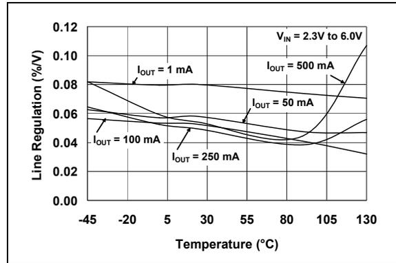
**FIGURE 2-4:** Line Regulation vs. Temperature (1.8V Adjustable).
