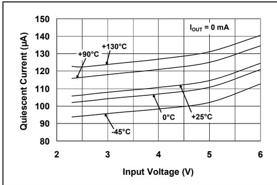
**FIGURE 2-1:** Quiescent Current vs. Input Voltage (1.8V Adjustable).
