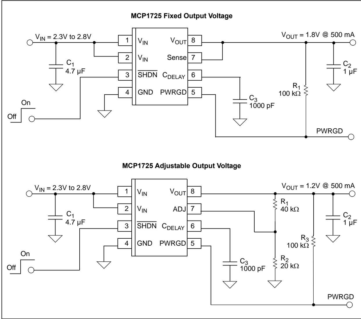
Functional Block Diagram - Adjustable Output
