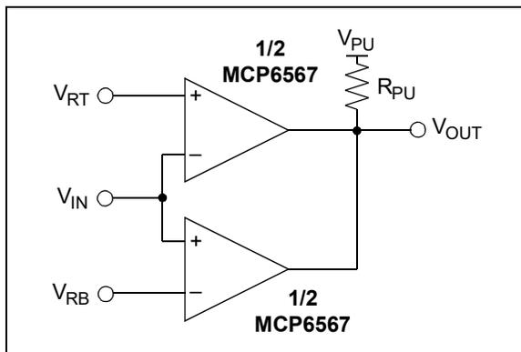
**FIGURE 4-13:** Windowed Comparator.
