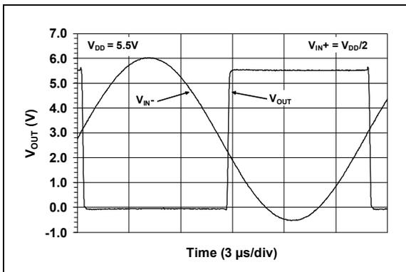
**FIGURE 2-3:** Input vs. Output Signal, No Phase Reversal.
