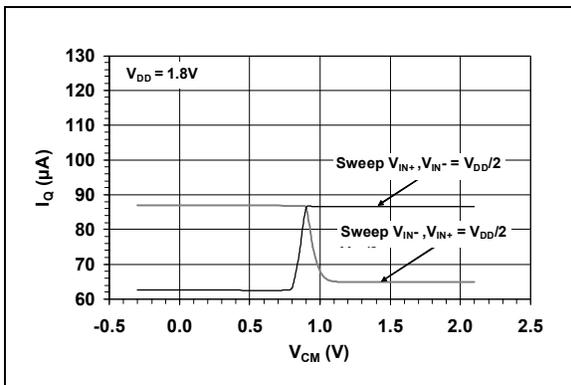
**FIGURE 2-15:** Quiescent Current vs. Common-mode Input Voltage.
