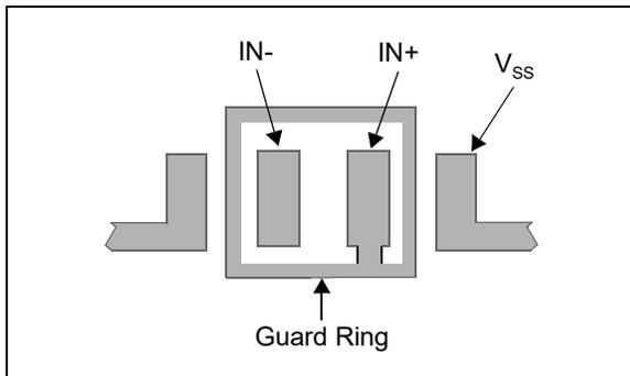
**FIGURE 4-9:** Example Guard Ring Layout for Inverting Circuit.
