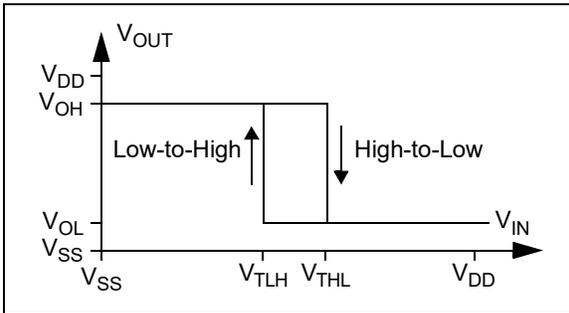
**FIGURE 4-7:** Hysteresis Diagram for the Inverting Circuit.
