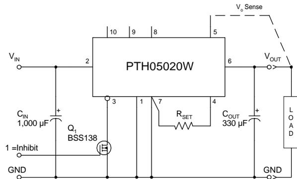
Turning  $Q_1$  on applies a low voltage to the *Inhibit* control and disables the output of the module. If  $Q_1$  is then turned off, the module will execute a soft-start power-up. A regulated output voltage is produced within 20 msec. Figure 3-4 shows the typical rise in both the output voltage and input current, following the turn-off of  $Q_1$ . The turn off of  $Q_1$  corresponds to the rise in the waveform,  $Q_1 V_{ds}$ . The waveforms were measured with a 5-A load.
