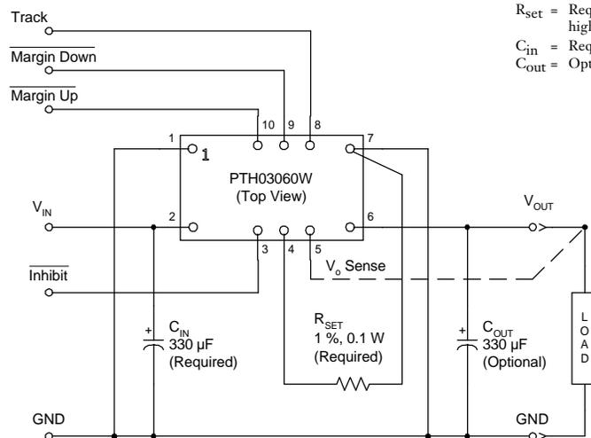
R<sub>set</sub> = Required to set the output voltage to a value higher than 0.8 V. (See spec. table for values)
