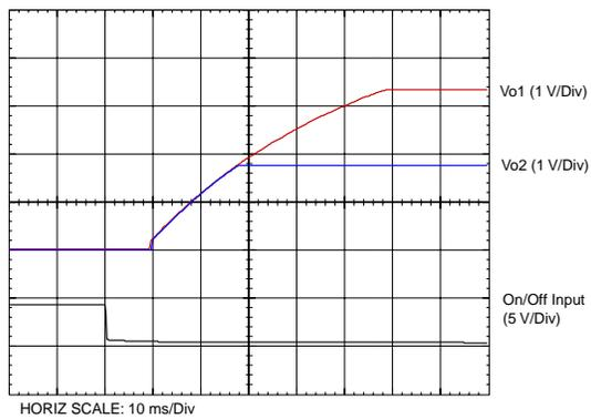
**Figure 3-7; Simultaneous Power Down with Auto-Track Control**
