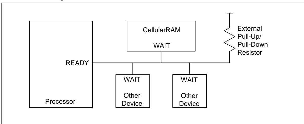
When a READ or WRITE operation has been initiated, WAIT goes active to indicate that the ADMUX PSRAM device requires additional time before data can be transferred. For READ operations, WAIT will remain active until valid data is output from the device. For WRITE operations, WAIT will indicate to the memory controller when data will be accepted into the ADMUX PSRAM device. When WAIT transitions to an inactive state, the data burst will progress on successive clock edges.
