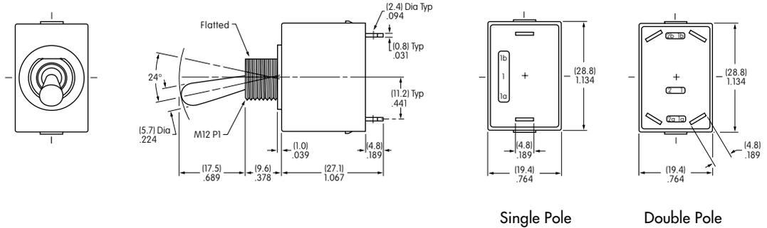
The .094" (2.4mm) diameter terminal hole accommodates one 12-gauge solid or stranded wire.
