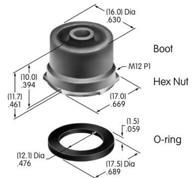
Note: When using boot assembly AT401, also use o-ring AT401P from the standard hardware supplied. Hex face nut AT503 & lockwasher AT508 are not used with boot assembly.
