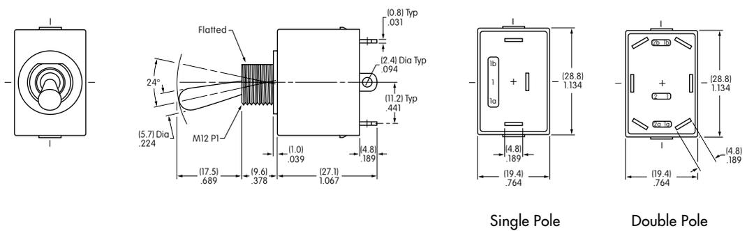
The .094" (2.4mm) diameter terminal hole accommodates one 12-gauge solid or stranded wire.
