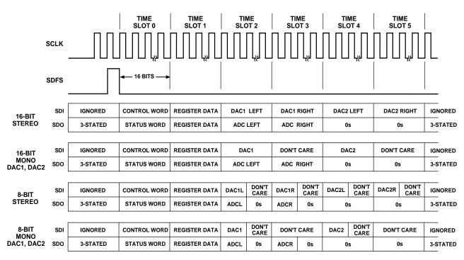
THE DIAGRAM ABOVE IS INTENDED TO BE ILLUSTRATIVE OF THE MORE COMMONLY USED CONFIGURATIONS. ADC LEFT, ADC RIGHT, DAC1 AND DAC2 CAN BE INDIVIDUALLY ASSIGNED TO 8-BIT OR 16-BIT SAMPLE WIDTH, AND DAC1 AND DAC2 CAN BE INDIVIDUALLY ASSIGNED TO STEREO OR MONO MODE. EACH AD1843 CONSUMES 6 TMD SLOTS (REQUIRING 96 SCLK PERIODS), LEAVING 10 TDM SLOTS UNUSED IN A 16 SLOT FRAME.
