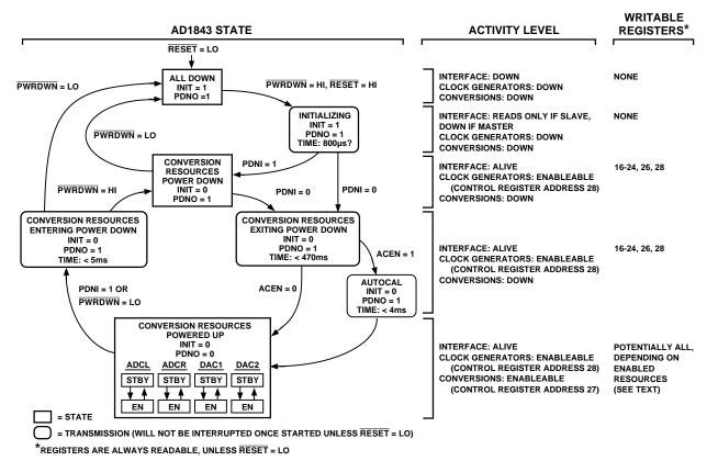
Figure 17. AD1843 Start-Up Sequence State Diagram
