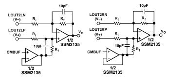
Figure 24. AD1843 Differential-to-Single-Ended Converter Line Output Connections
