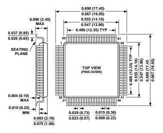
ST-100 100-Terminal Plastic Thin Quad Flatpack (TQFP)
