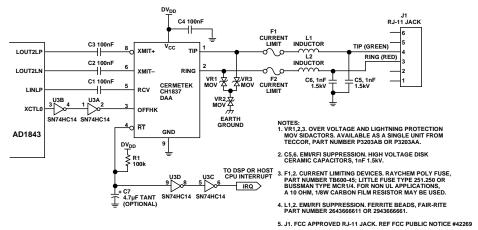
Figure 32. Cermetek DAA Example Circuit
