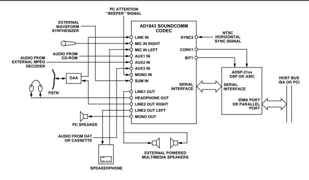
Figure 6. Typical Configurations
