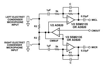
Figure 22. AD1843 "Phantom-Powered" Microphone Input Circuit
