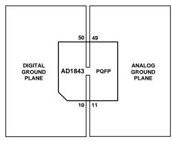
Figure 35a. AD1843 Recommended PQFP Ground Plane
