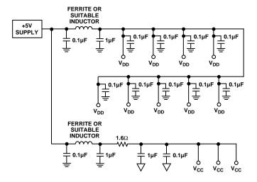
Figure 33. AD1843 Recommended Power Supply Bypassing
