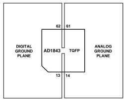
Figure 35b. AD1843 Recommended TQFP Ground Plane
