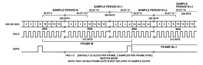
Figure 7. FRS = 0, Master Mode Timing
