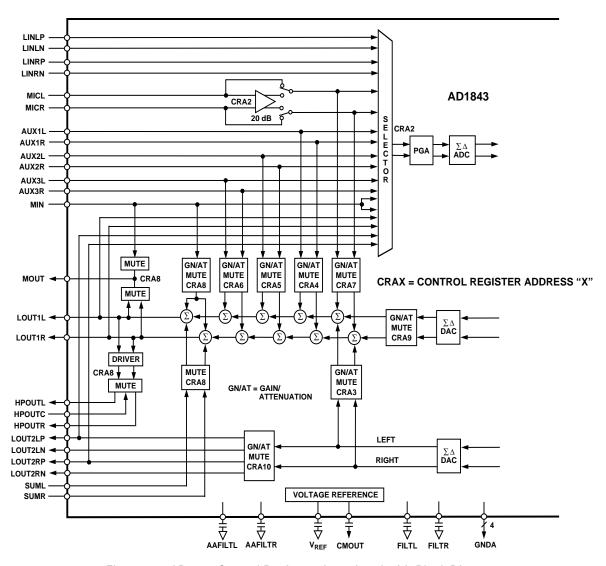
Figure 12. AD1843 Control Registers Associated with Block Diagram
