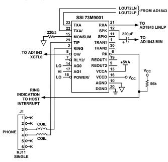
Figure 31. Silicon Systems DAA Example Circuit
