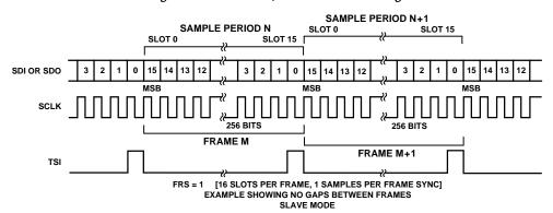
Figure 10b. FRS = 1, Slave Mode Timing
