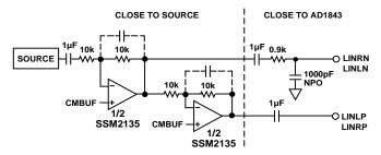
Figure 21. Single-Ended to Differential Converter
