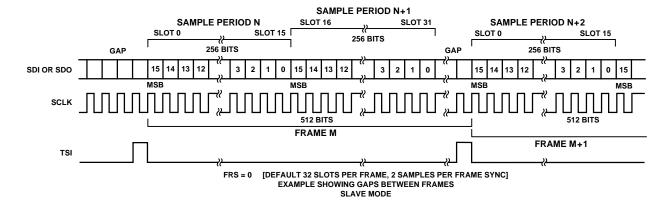
Figure 9a. FRS = 0, Slave Mode Timing
