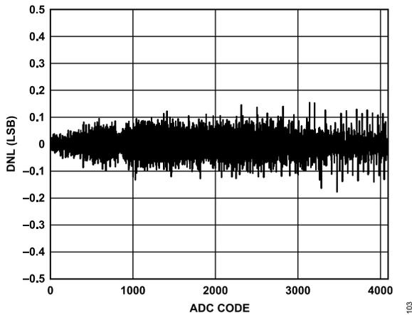
Figure 12. ADC DNL,  $V_{DD} = 5.5\text{ V}$
