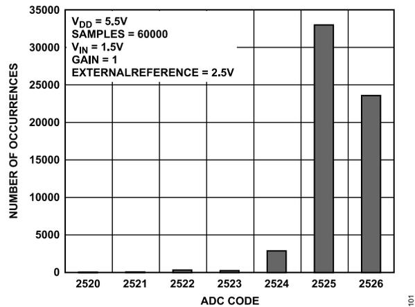
Figure 16. Histogram of ADC Codes,  $V_{DD} = 5.5\text{ V}$
