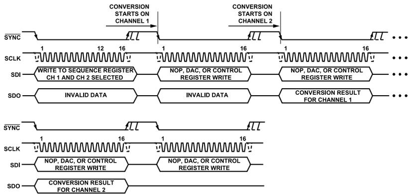
Figure 47. Multichannel ADC Conversion Sequence, No Repeat
