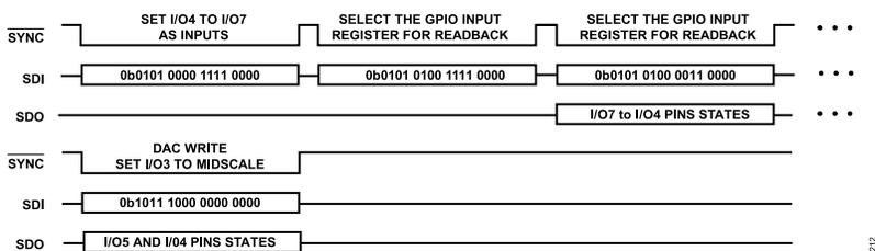
Figure 50. Configuring and Reading General-Purpose Input Pins
