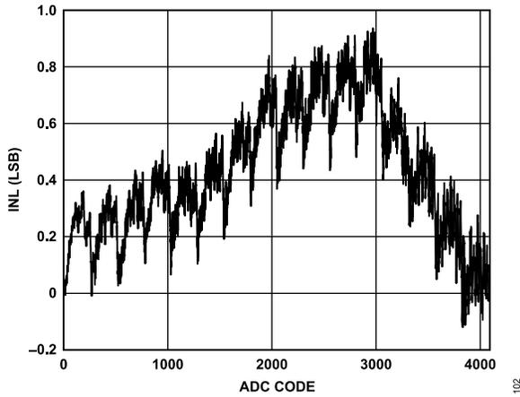
Figure 11. ADC INL,  $V_{DD} = 5.5\text{ V}$
