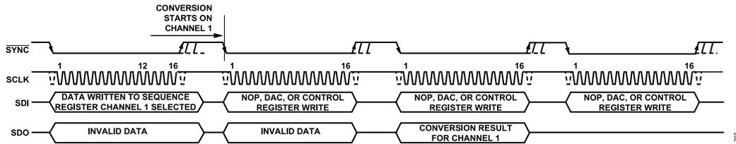
Figure 45. Single-Channel ADC Conversion Sequence, No Repeat
