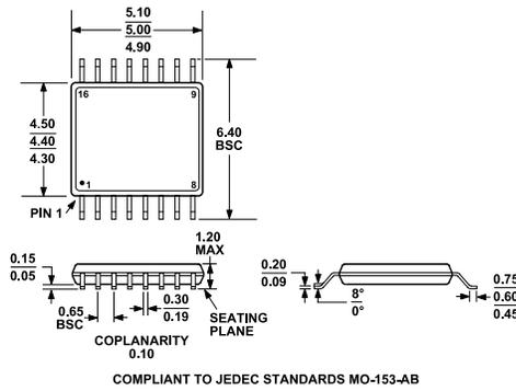
Figure 53. 16-Lead Thin Shrink Small Outline Package [TSSOP] (RU-16)
