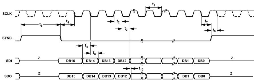
**Figure 4. Serial Read and Write Timing Diagram**
