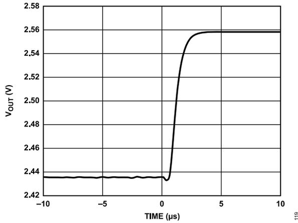
Figure 23. DAC Settling Time (100 Code Change, Rising Edge)
