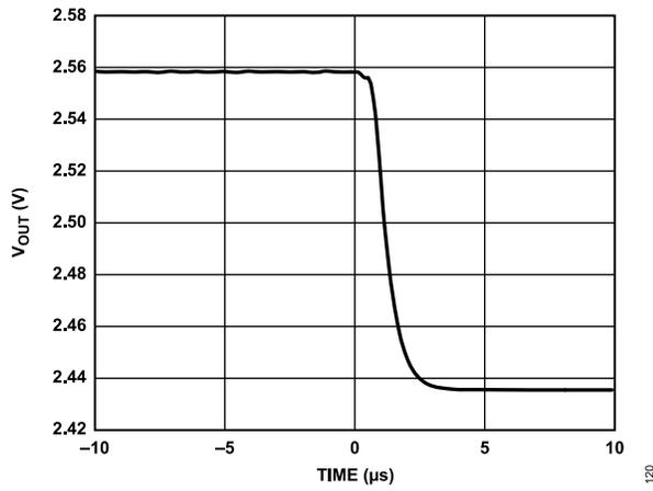
Figure 24. DAC Settling Time (100 Code Change, Falling Edge)
