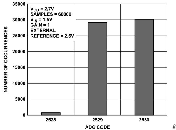
Figure 15. Histogram of ADC Codes,  $V_{DD} = 2.7\text{ V}$
