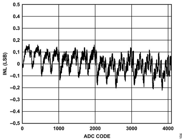
Figure 13. ADC INL,  $V_{DD} = 2.7\text{ V}$
