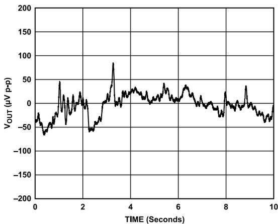
Figure 31. DAC 1/f Noise with Internal Reference
