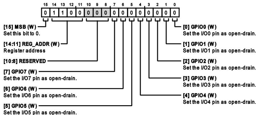
Table 26. Bit Descriptions for GPIO\_OPENDRAIN\_CONFIG
