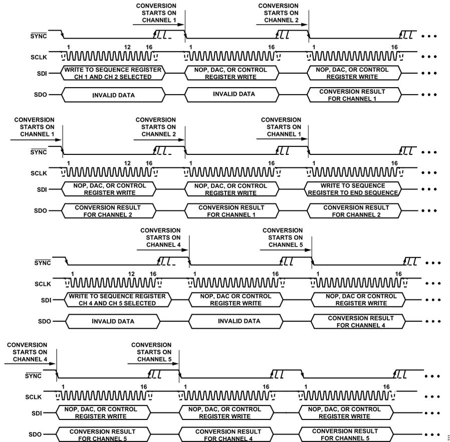
Figure 49. Changing a Multichannel, Repeating, ADC Conversion Sequence
