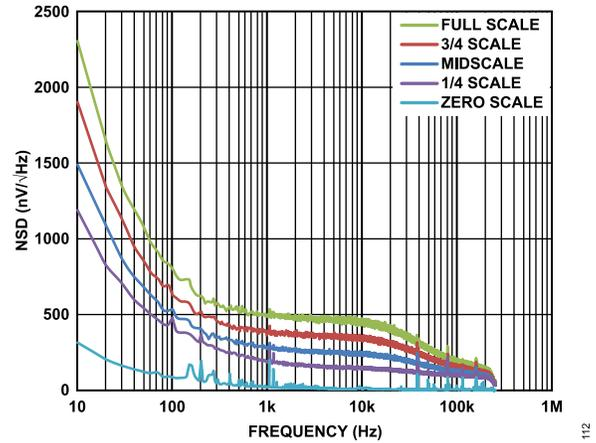
Figure 32. DAC Output Noise Spectral Density (NSD)
