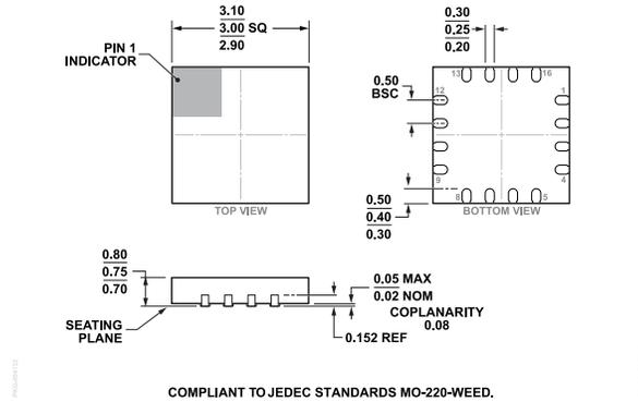
Figure 54. 16-Lead Lead Frame Chip Scale Package [LFCSP] 3 mm x 3 mm Body, Very Very Thin Quad (CP-16-32)
