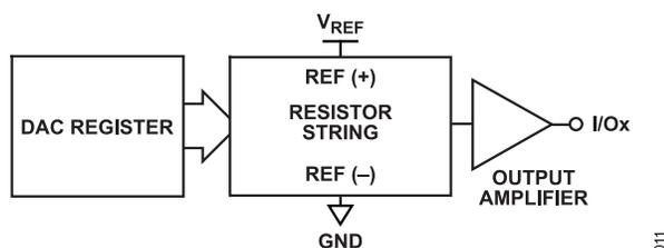
Figure 38. Internal Block Diagram of the DAC Architecture
