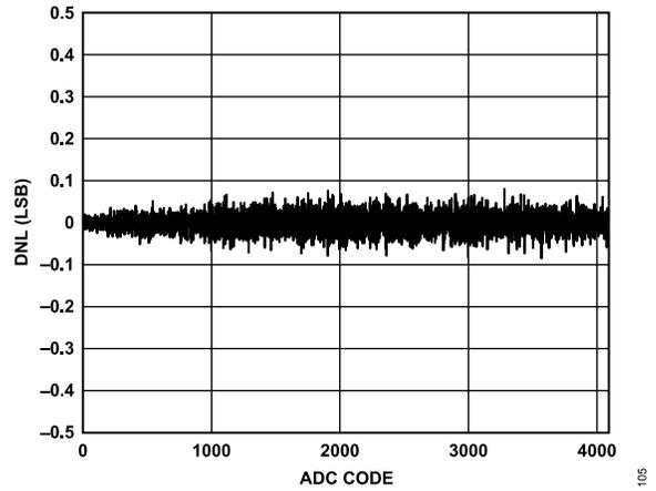
Figure 14. ADC DNL,  $V_{DD} = 2.7\text{ V}$
