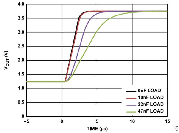
Figure 27. DAC Settling Time for Various Capacitive Loads
