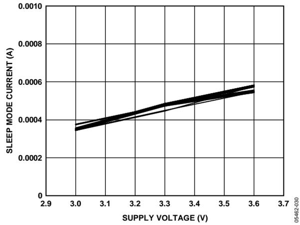
Figure 30. Sleep Mode Current vs. Supply at 25°C
