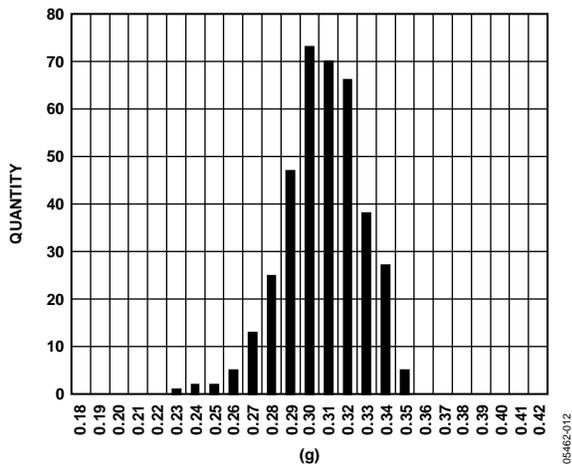
Figure 12. Y-Axis Self-Test Level at 25°C/3.3 V
