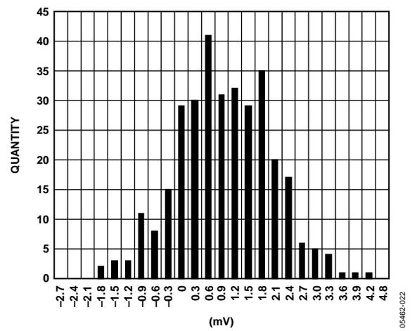
Figure 22. DAC Offset Distribution at 25°C/3.3 V
