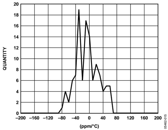
Figure 15. Inclination Offset Tempco Histogram at 3.3 V
