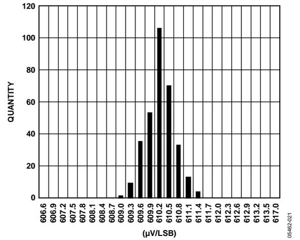
Figure 21. DAC Gain Distribution at 25°C/3.3 V
