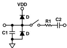
Figure 35. Equivalent Analog Input Circuit
