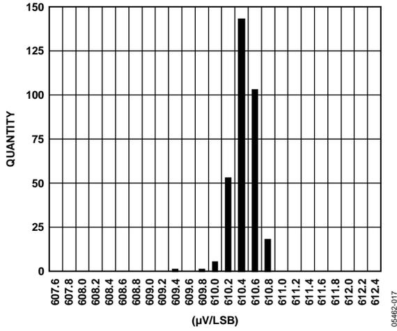
Figure 17. ADC Gain Distribution at 25°C/3.3 V
