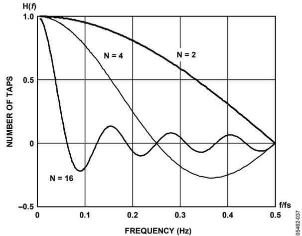
Figure 34. Number of Taps vs. Sample Frequency Response
