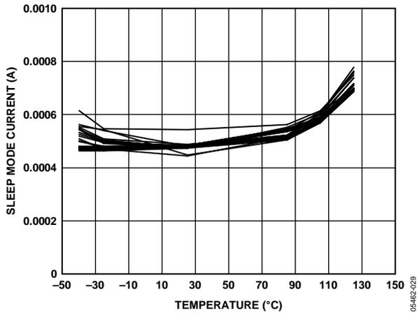
Figure 29. Sleep Mode Current vs. Temperature at 3.3 V
