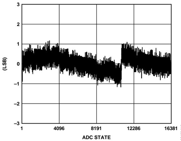
Figure 19. Typical ADC Integral Nonlinearity at 25°C/3.3 V
