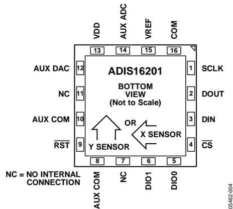
Figure 4. Pin Configuration
