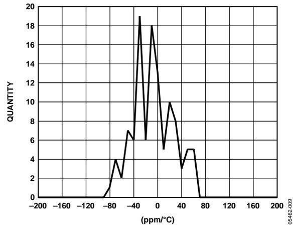
Figure 9. Acceleration Offset Tempco Histogram at 3.3V
