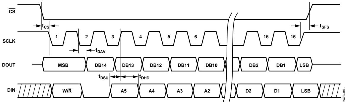
Figure 3. SPI Timing
