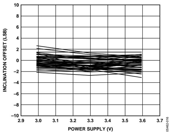
Figure 16. Inclination Offset vs. Supply at 25°C
