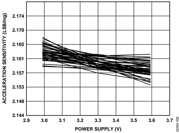
Figure 5. Acceleration Sensitivity vs. Power Supply at 25°C
