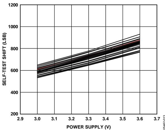
Figure 13. Self-Test Shift vs. Supply at 25°C
