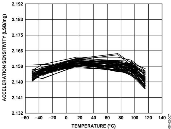
Figure 7. Acceleration Sensitivity vs. Temperature at 3.3V
