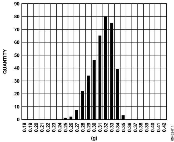
Figure 11. X-Axis Self-Test Level at 25°C/3.3 V
